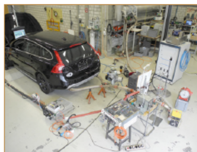
Figure 3 (left): Mobile Smog chamber of the PSI to study SOA formation of GDI vehicle exhausts.
