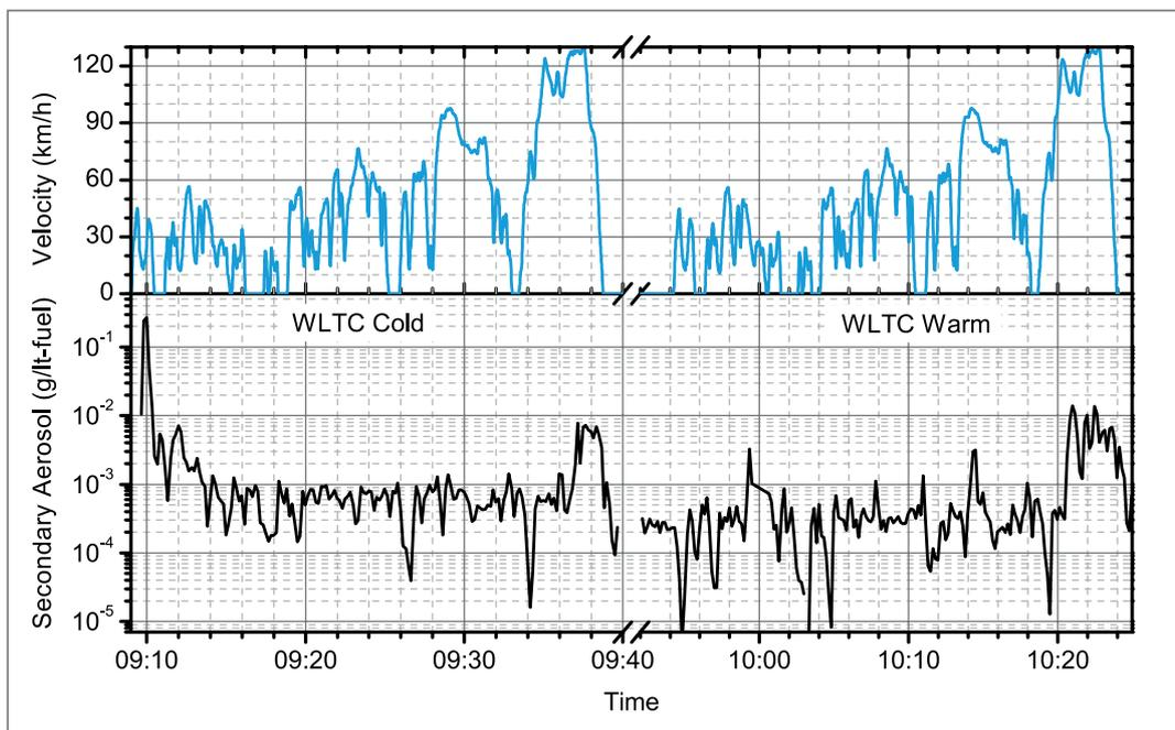
Figure 4 : Time-resolved SOA potential (logarithmic scale), obtained using the micro-smog chamber, during cold and hot WLTC for an Euro-5 vehicle (Volvo, V60, 1.6 L). The mass concentration was derived from the observed number concentration, average mass distributions from the SSC, and a particle density  $\rho = 2000 \text{ kg/m}^3$ .
