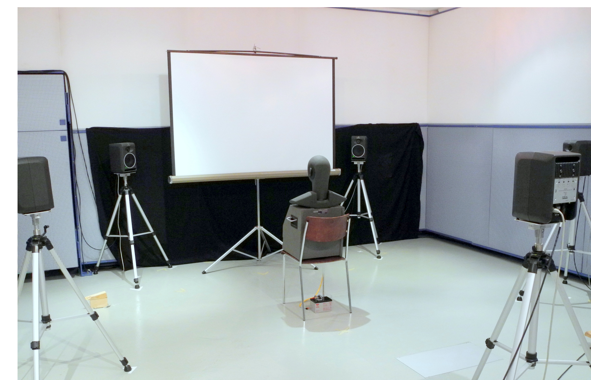
Figure 4: Sound reproduction setup of a previous experiment at Empa. The setup was used in an experiment to determine what Ambisonics decoding strategy to use considering how the head of the listener perturbs the sound field.
