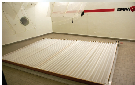
Figure 1: Reverberation chamber at Empa with a curtain mounted with 100% fullness
