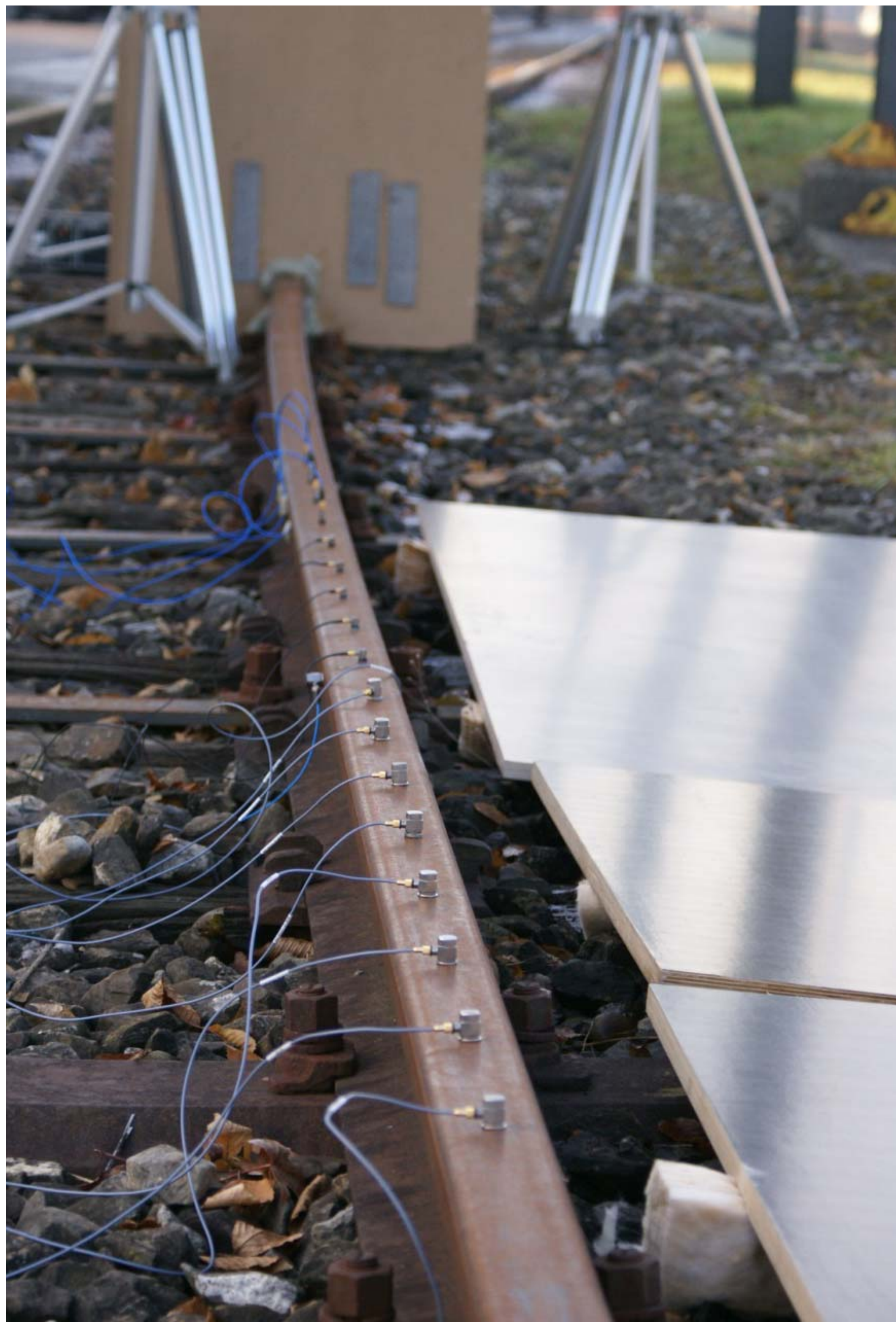
Figure 1: Experimental determination of acoustical track transfer function
