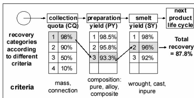
Figure 3 Method used to assess the product-specific recycling quota for construction parts that are made from Aluminium.
