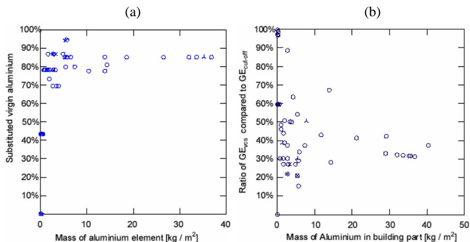
Figure 4 Results showing the influence of the mass of the construction part on the overall results of (a) substitution and (b) the indicator "Graue Energie". Small parts are merely not collected and lost. Overlaying data points are represented with a symbol with more strokes (cross, star, etc.).
