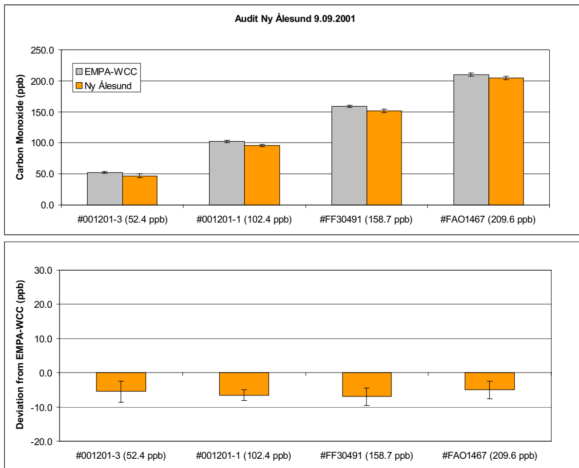
Figure 12: upper panel: concentrations of the WCC transfer standards (grey, reference: CMDL CA02859, 194.7 ppb) measured with the GC system of the Zeppelin station (orange). lower panel: deviation of Zeppelin station from the conventional true value.
