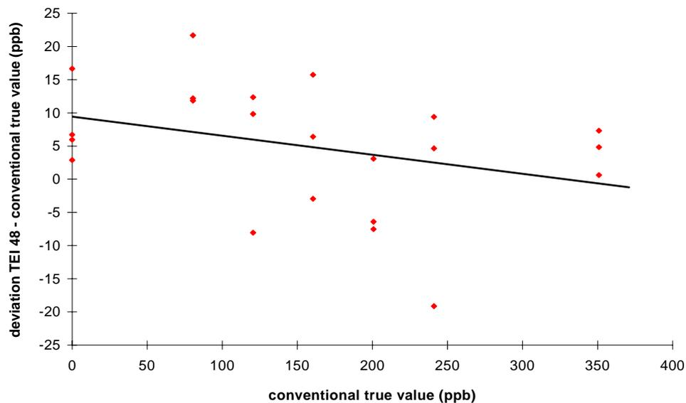
Figure 2: Intercomparison of CO instrument TEI 48
