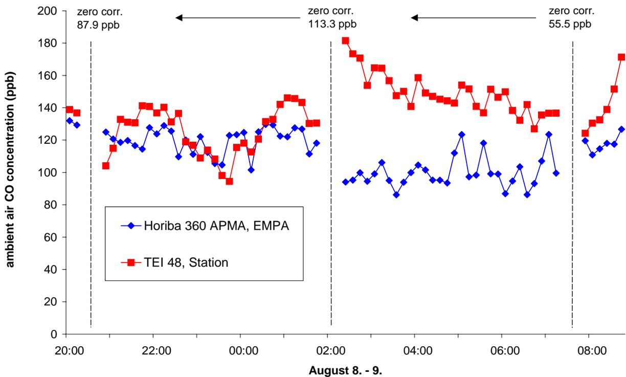
Figure 16: Ambient air concentrations during 2. night, measured with the field instrument TEI 48 and the transfer standard Horiba 360 APMA, by-passing the cooling trap
