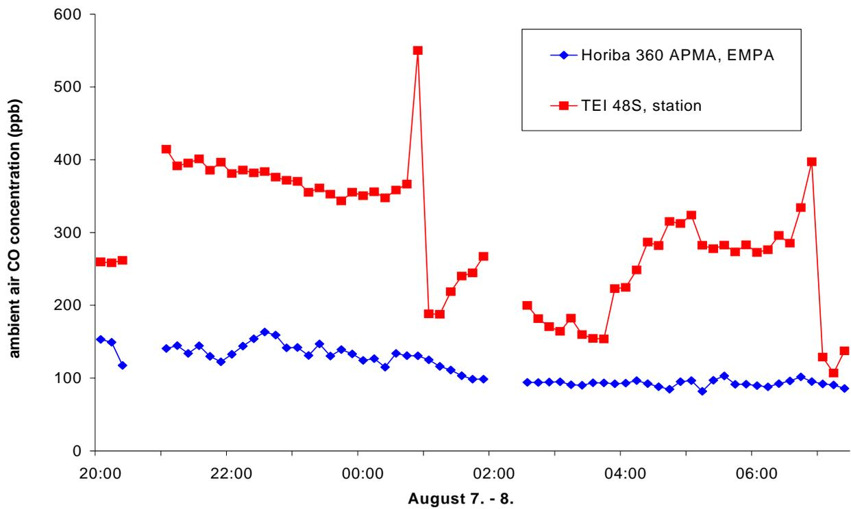
Figure 15: Ambient air concentrations during 1. night, measured with the field instrument TEI 48 and the transfer standard Horiba 360 APMA, leakage in the cooling trap of the station
