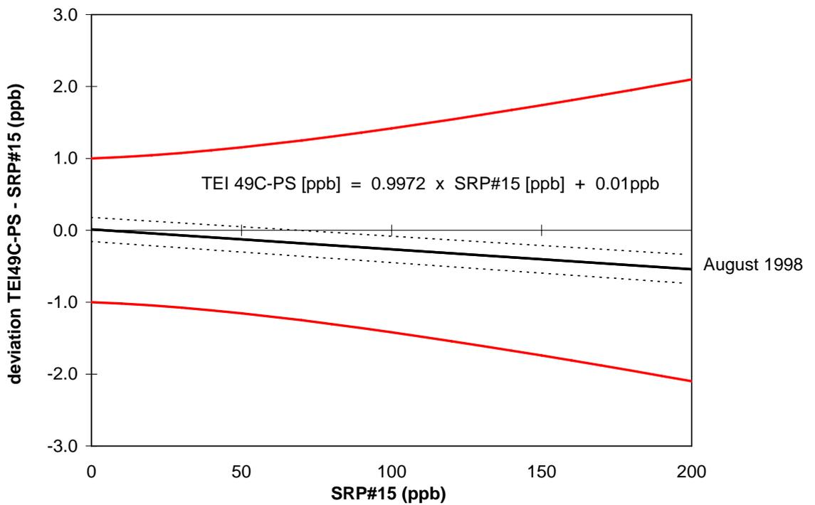
Figure 20: Transfer standard (O<sub>3</sub>) after audit
