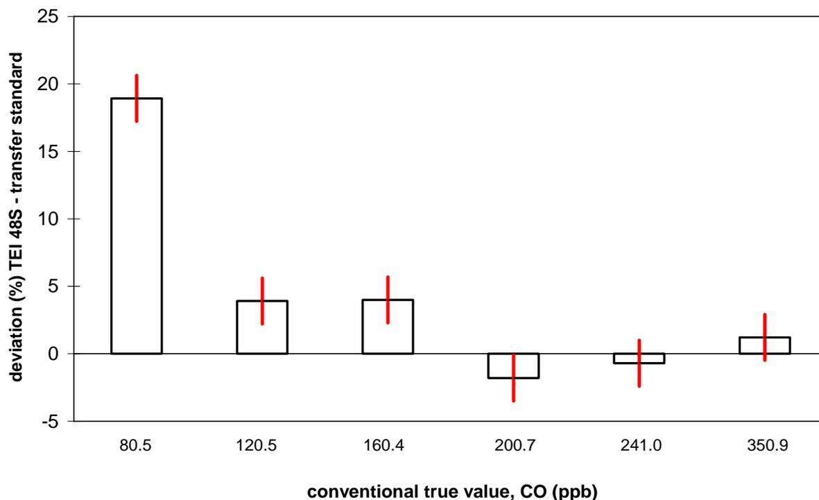
Figure 14: Differences (%) between TEI 48 and the transfer standard (the red lines show the whole uncertainty of the audit procedure)
