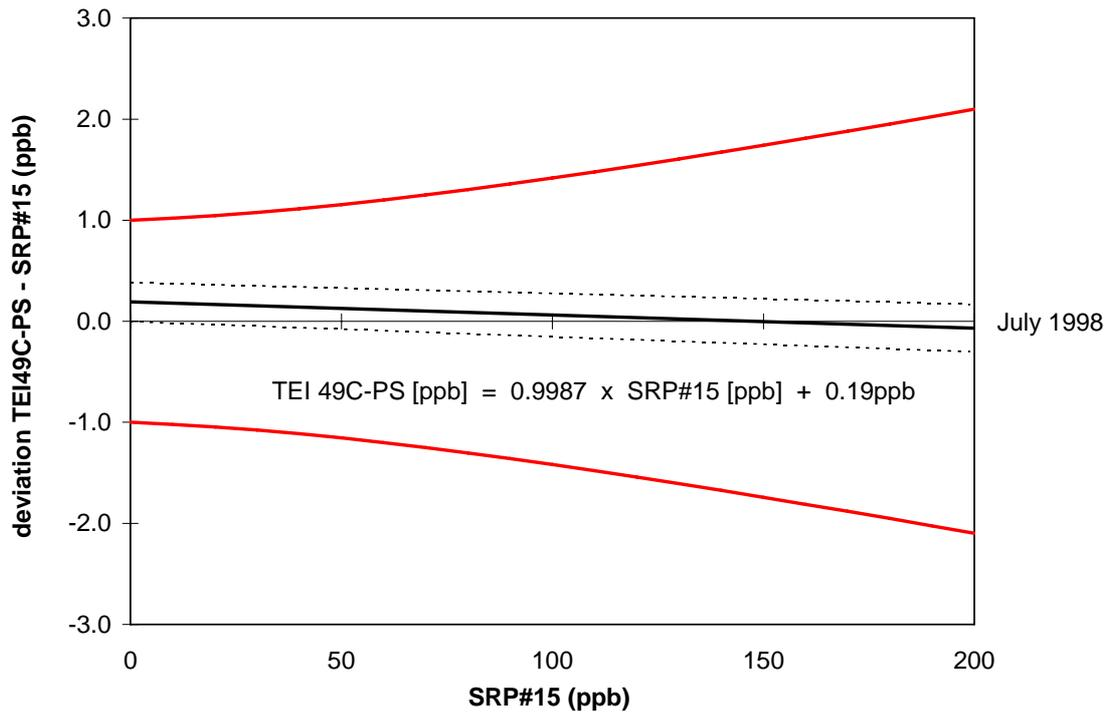
Figure 19: Transfer standard (O<sub>3</sub>) before audit
