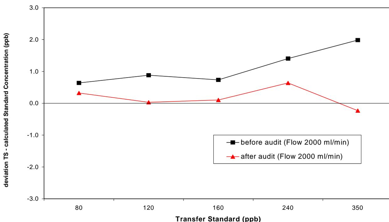
Figure 22: Transfer standard (MGM diluter) before and after audit.
