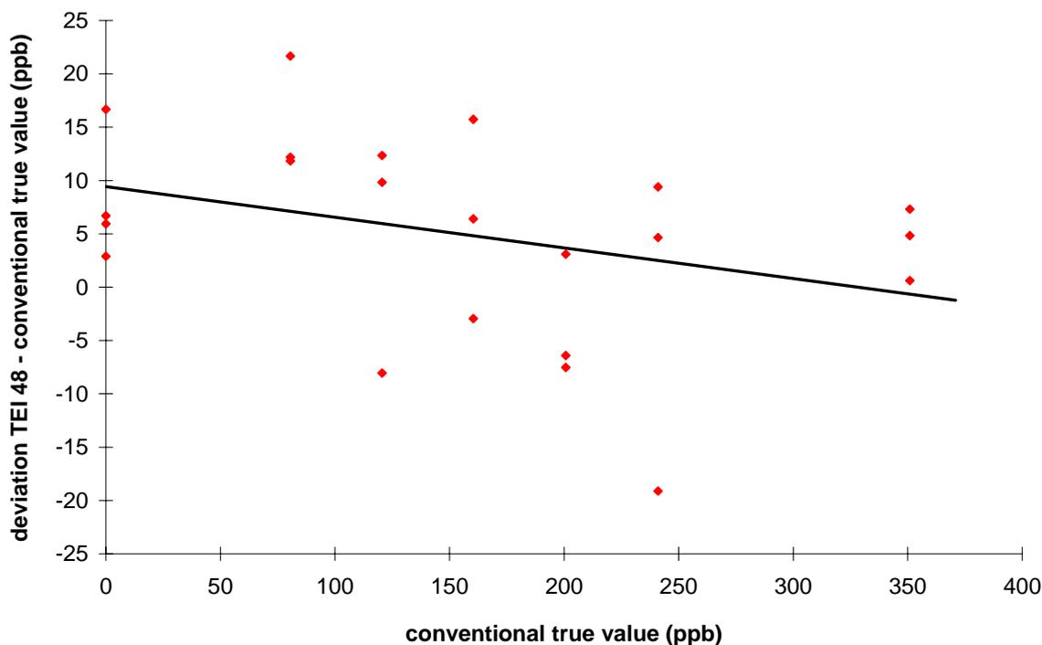
Figure 13: Differences (ppb) between the TEI 48 and the transfer standard
