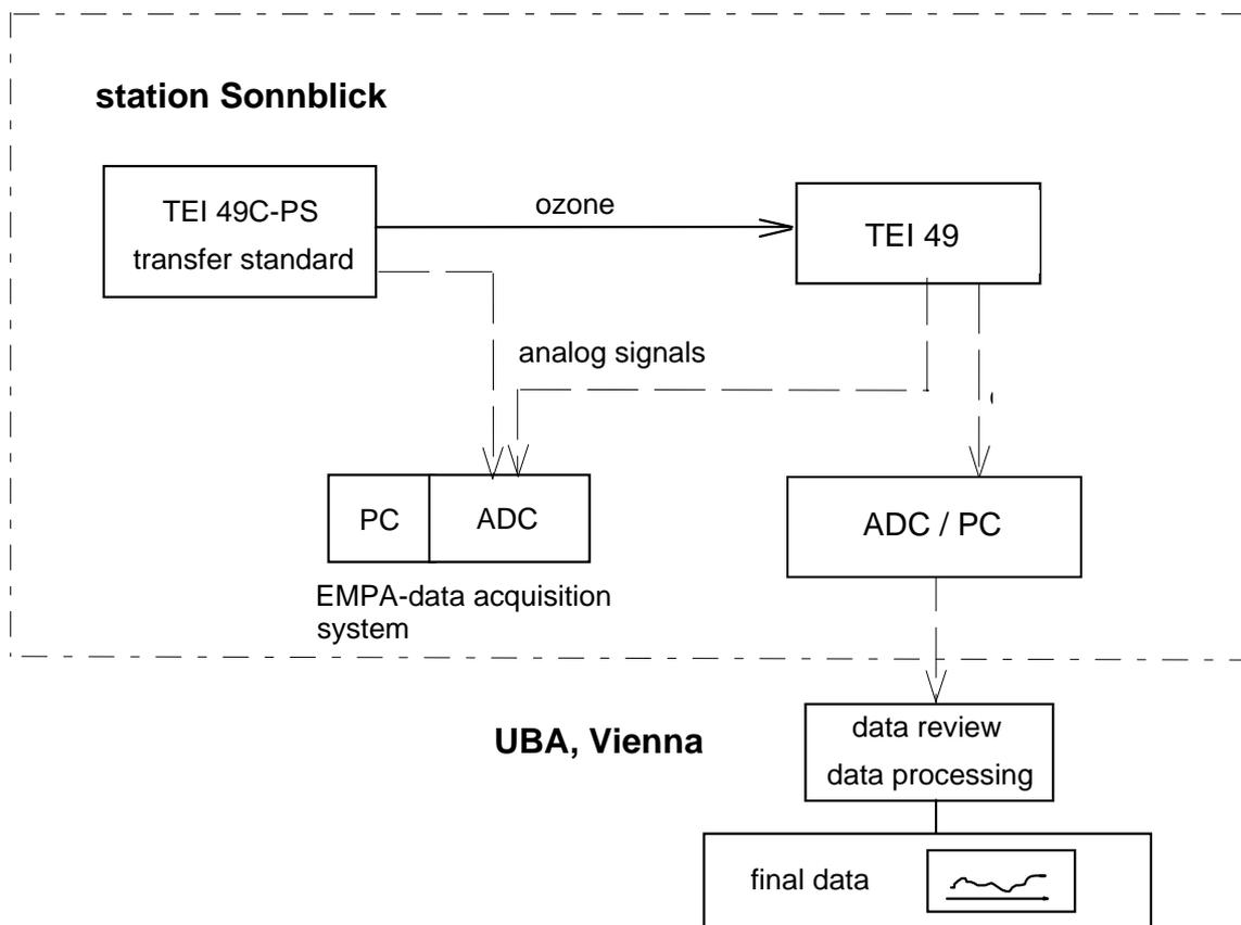
Figure 7: Experimental set up, ozone
