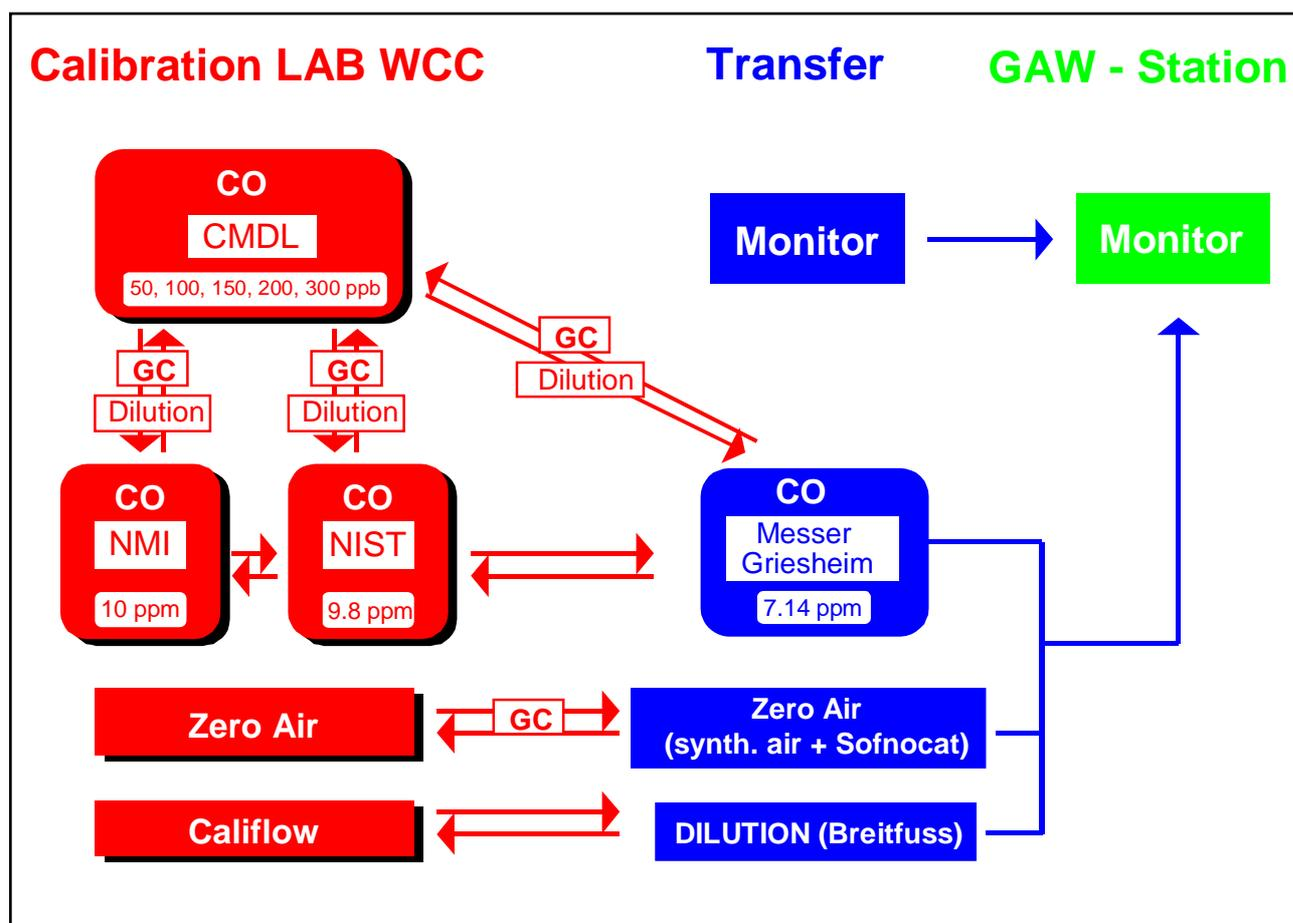
Figure 21: Traceability chain of the carbon monoxide audit.
