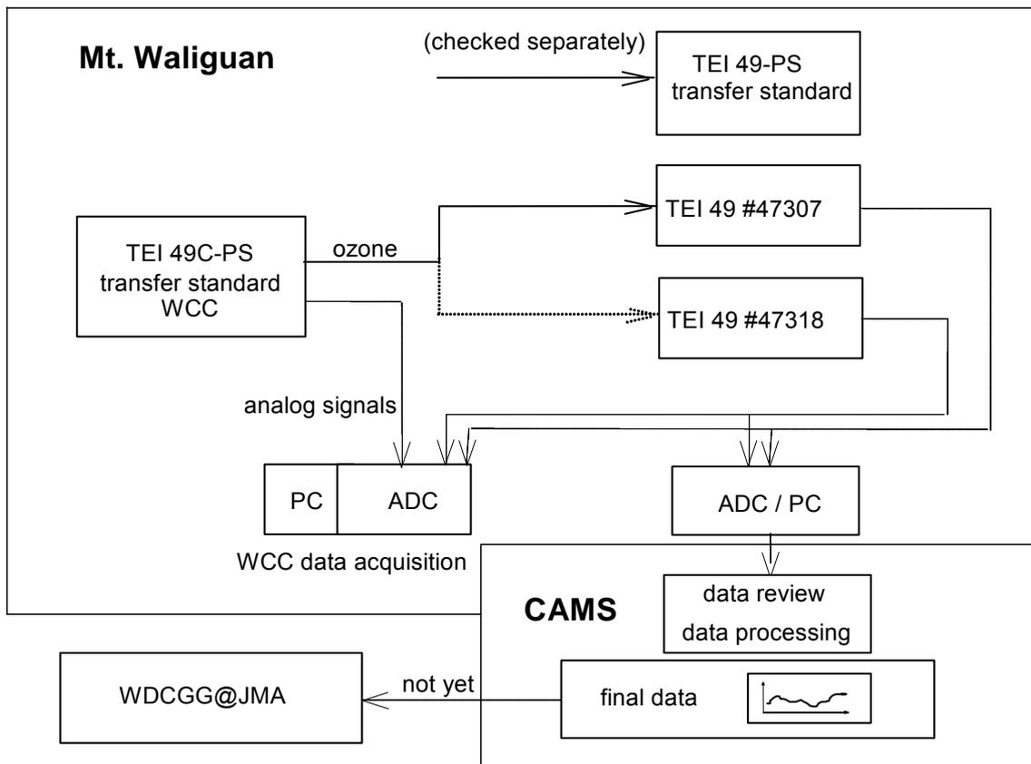
Figure 10: Experimental set up for the ozone inter-comparison
