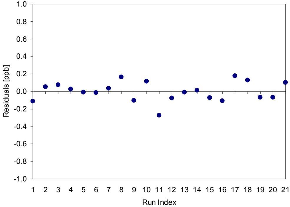
Figure 11: Residuals to the linear regression function (TEI 49 #47318-278) vs. the run index (time dependence)
