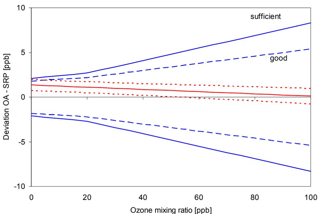
Figure 1: Inter-comparison of instrument TEI 49 #47318-278
