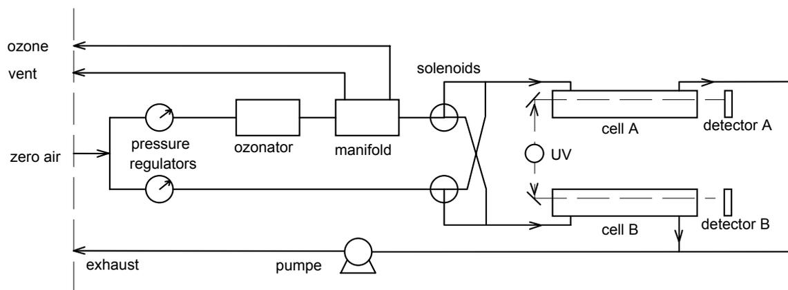
Figure 24: Flow schematic of TEI 49C-PS
