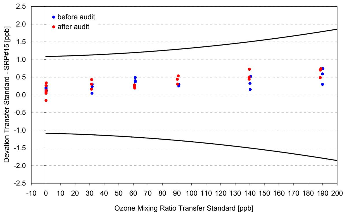
Figure 26: Deviation of the WCC-Empa transfer standard from SRP#15 before and after the audit
