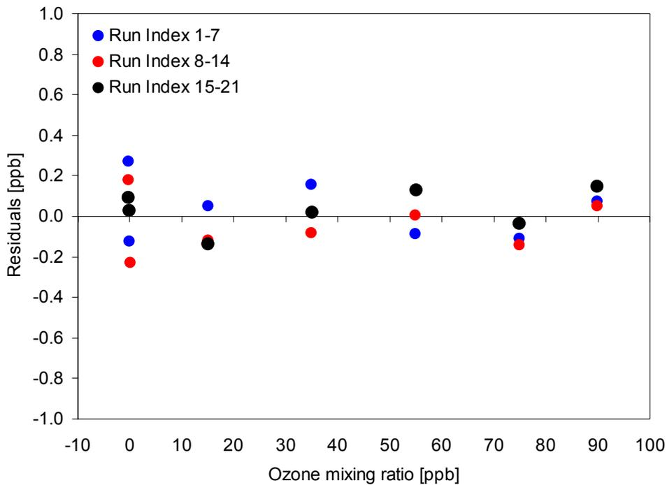
Figure 15: Residuals to the linear regression function (TEI 49 #47307-278) vs. the concentration of the WCC transfer standard (concentration dependence)
