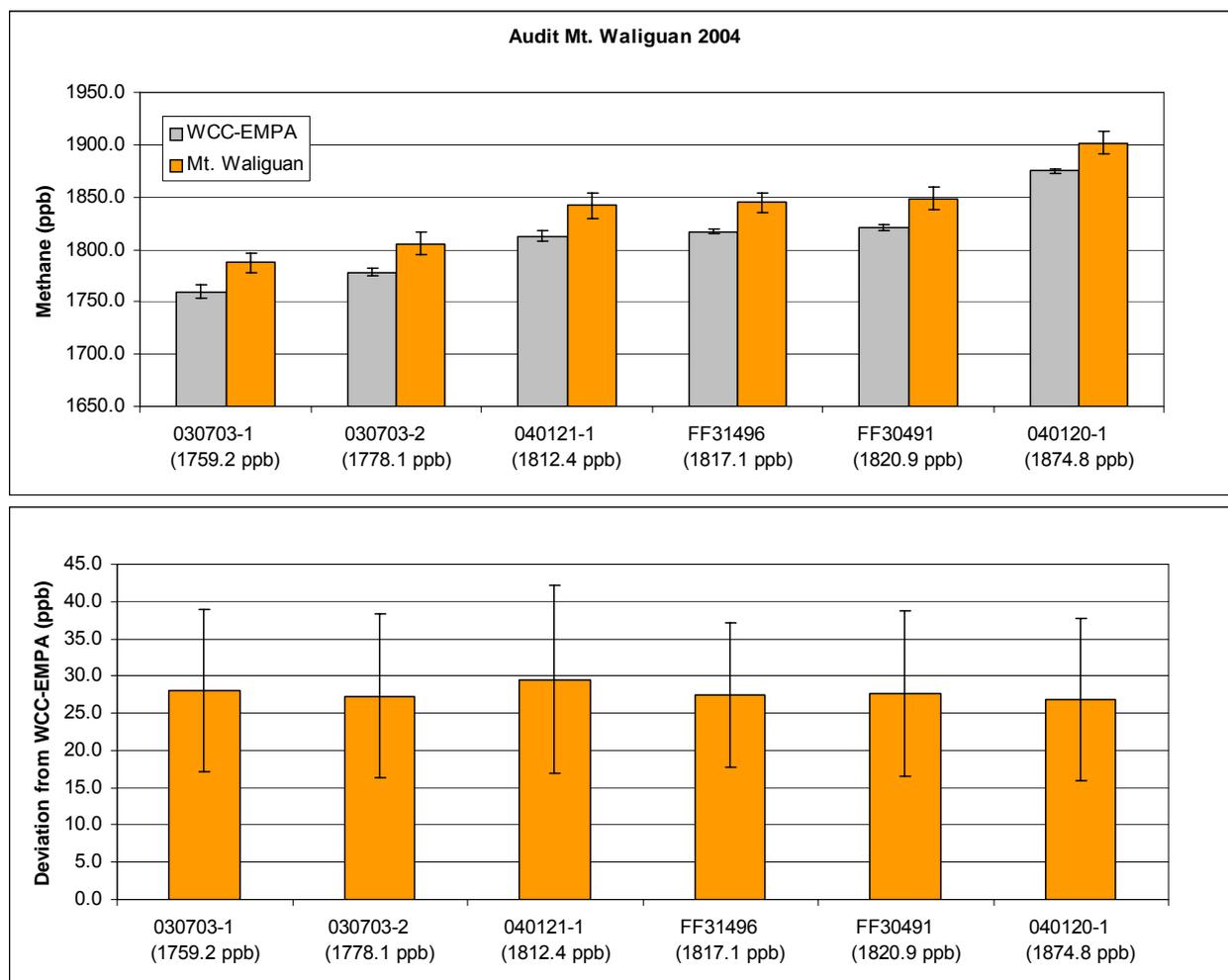
Figure 23: upper panel: concentrations of the WCC transfer standards (grey, reference: CMDL scale, Appendix IV) measured with the GC system of Mt. Waliguan (orange, reference: MSC scale).
