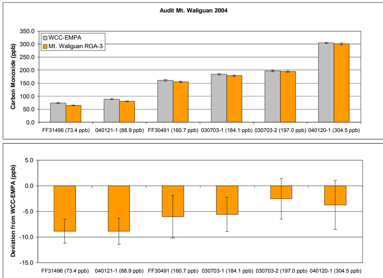
Figure 3: upper panel: concentrations of the WCC transfer standards (grey, reference: CMDL CA02854, 295.5 ppb) measured with the GC system of Mt. Waliguan (orange). lower panel: deviation of the Mt. Waliguan station from the reference. The error bars represent the 95% confidence interval.
