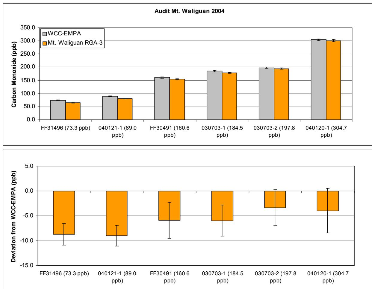
Figure 21: upper panel: concentrations of the WCC transfer standards (grey, reference: CMDL CA02854, 295.5 ppb) measured with the GC system of Mt. Waliguan (orange). lower panel: deviation of the Mt. Waliguan station from the reference. The error bars represent the 95% confidence interval.
