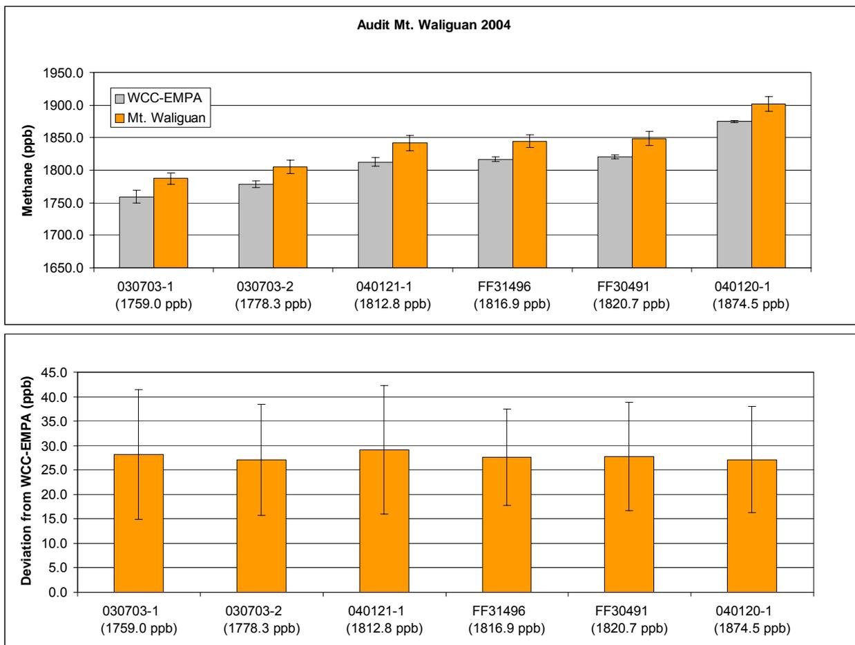
Figure 4: upper panel: concentrations of the WCC transfer standards (grey, reference: CMDL scale, Appendix IV) measured with the GC system of Mt. Waliguan (orange, reference: MSC scale). lower panel: deviation of Mt. Waliguan from the reference. The error bars represent the 95% confidence interval.
