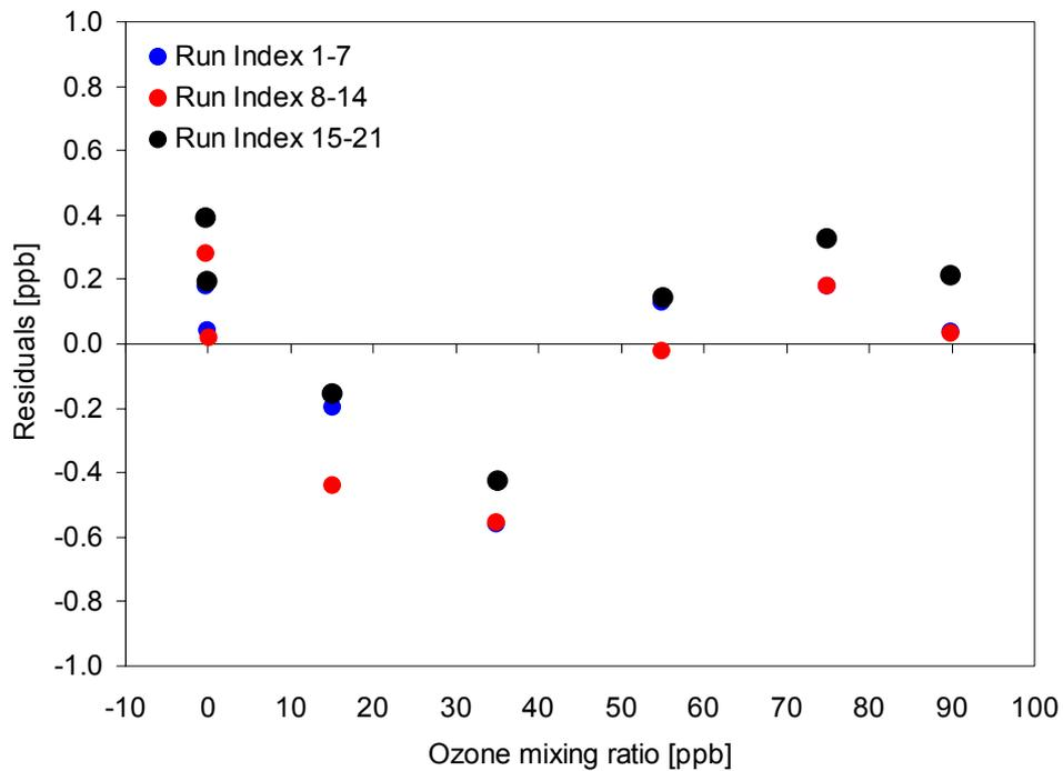
Figure 18: Residuals to the linear regression function (TEI 49PS #47651-279) vs. the concentration of the WCC transfer standard (concentration dependence)
