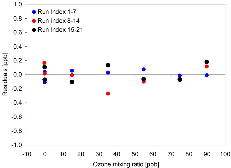
Figure 12: Residuals to the linear regression function (TEI 49 #47318-278) vs. the concentration of the WCC transfer standard (concentration dependence)
