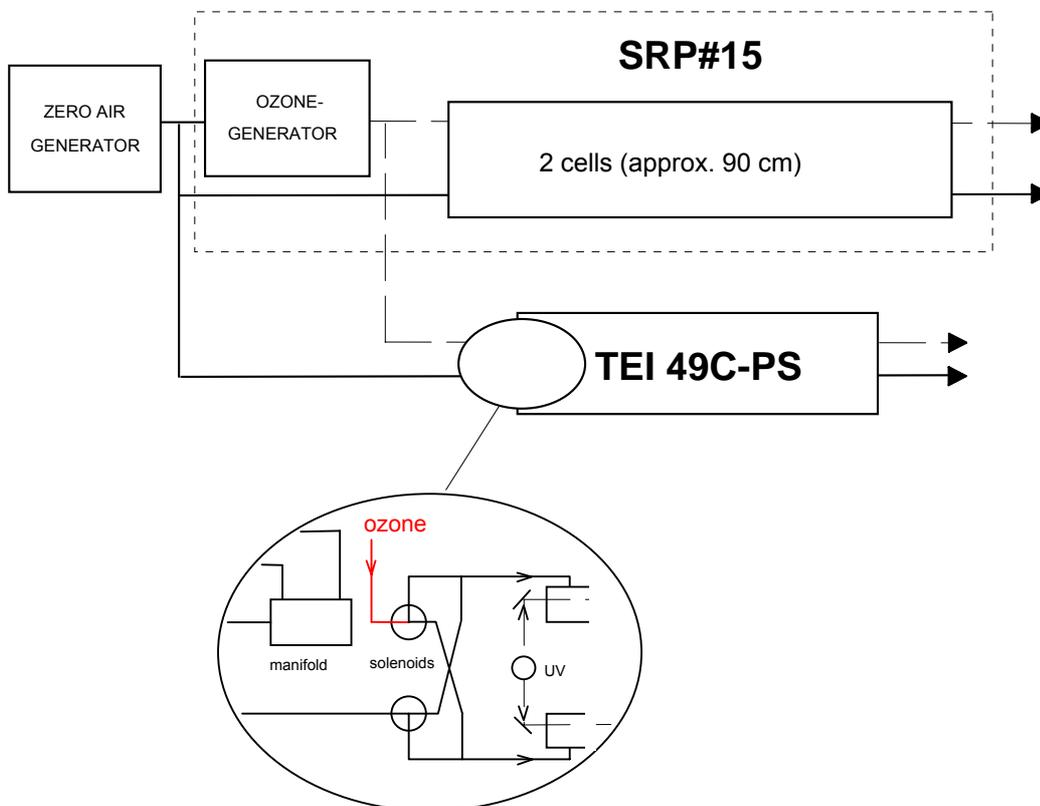
Figure 25: Instruments set up SRP -TEI 49C-PS
