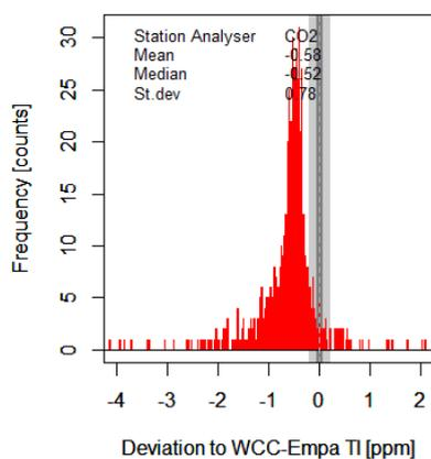
**Figure 15.** Deviation histograms for the LAU CO<sub>2</sub> NDIR analyser. 1 h data is shown for the station analyser – TI.
