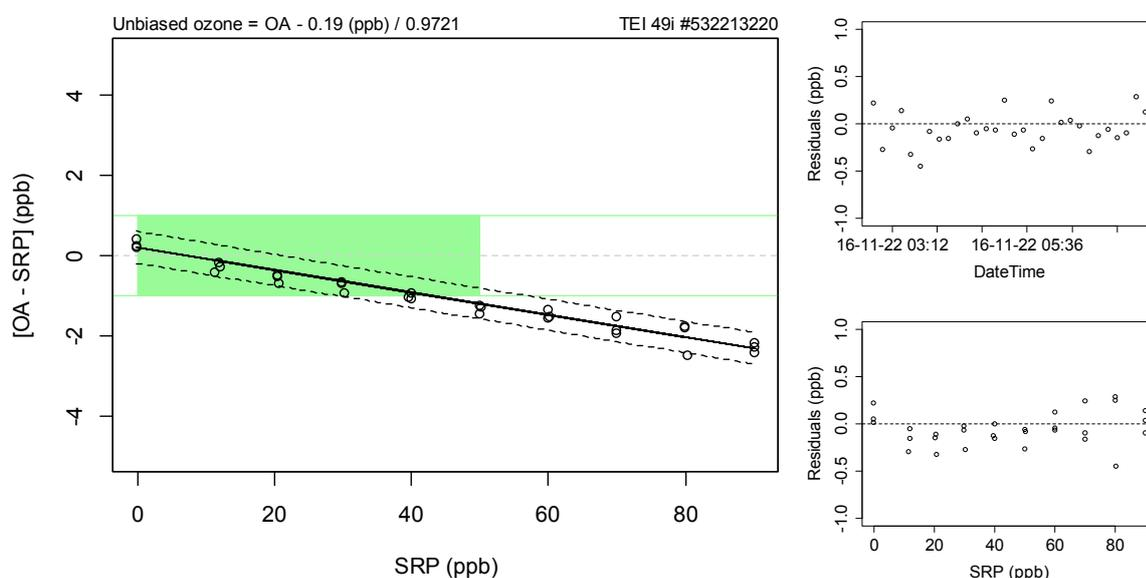
**Figure 2.** Same as above for the BHD ozone analyser (Thermo Scientific 49C #0532213220).
