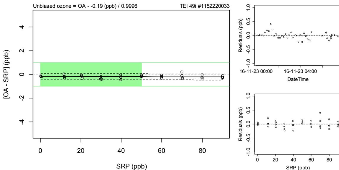
**Figure 4.** Same as above for the future BHD ozone analyser with final calibration settings (Thermo Scientific 49C #01152220033).
