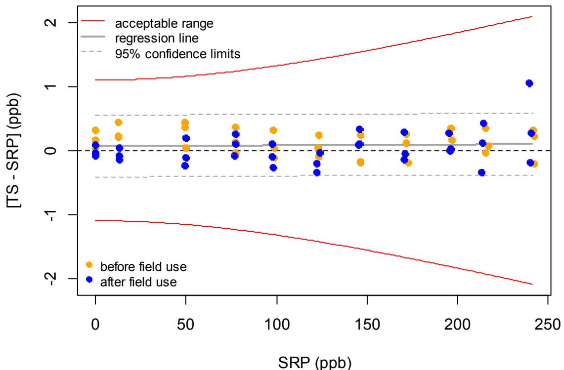
**Figure 18.** Deviations between traveling standard (TS) and Standard Reference Photometer (SRP) before and after use of the TS at the field site.
