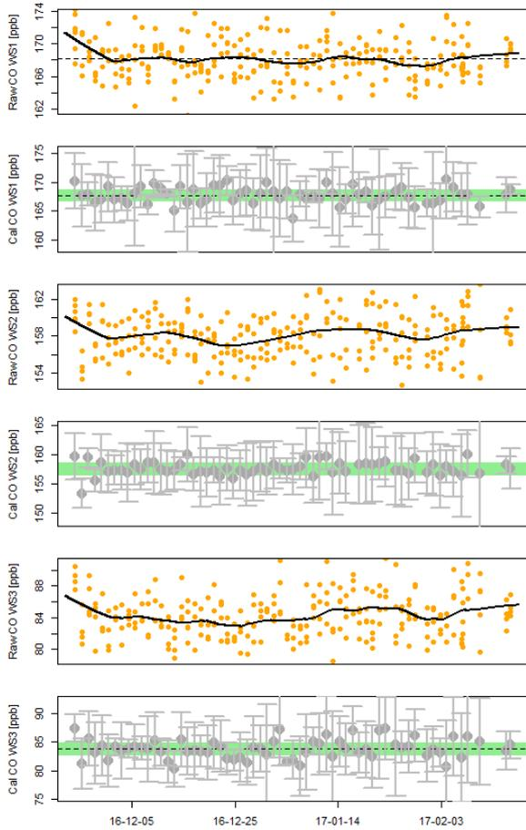
**Figure 21.** CO calibrations of the WCC-Empa-TI. The panels with the orange dots show raw 1 min values of the working standards and the loess fit (black line) used to account for drift. The other panels show the variation of the WS after applying the drift correction. Individual points in these panels are 5 min averages, and the error bars represent the standard deviation. The green area represents half of the WMO/GAW compatibility goals.
