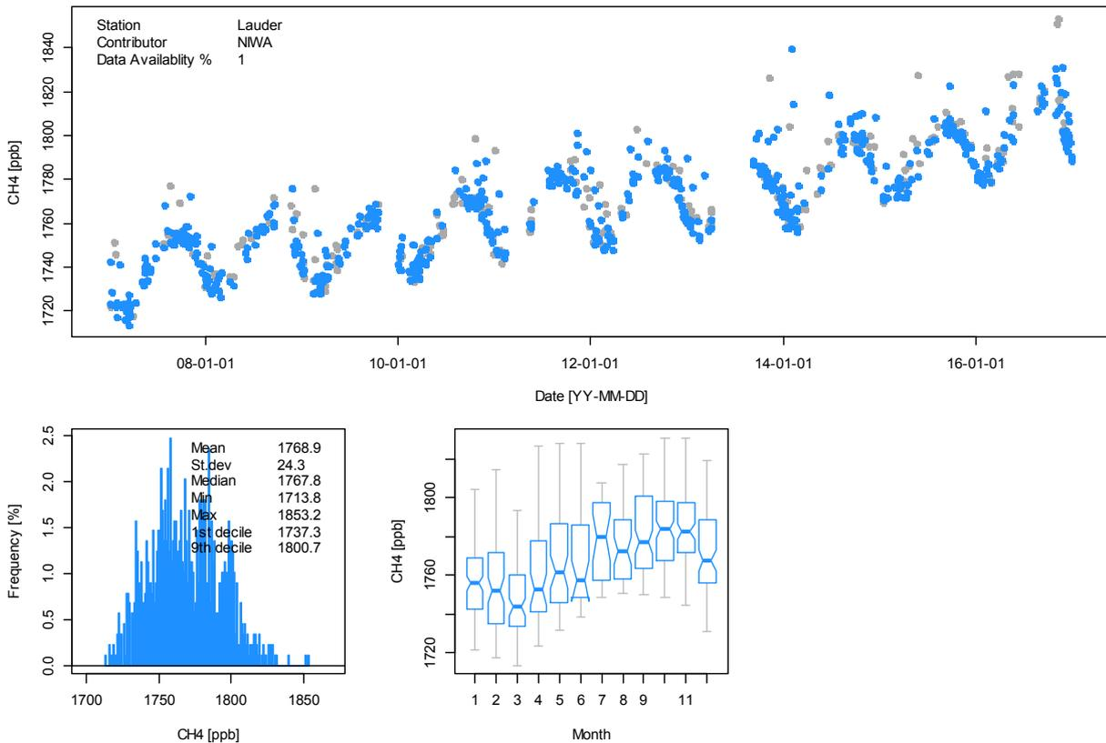
**Figure 16.** CH<sub>4</sub> data accessed from WDCGG. Top: Time series, hourly average for 3-4 pm local time. Blue dots are for wind speed >5 m/s, which is considered to be representative of well-mixed tropospheric air. Bottom: Left: Frequency distribution. Right: Seasonal variation; the horizontal blue line denotes to the median, and the blue boxes show the inter-quartile range.
