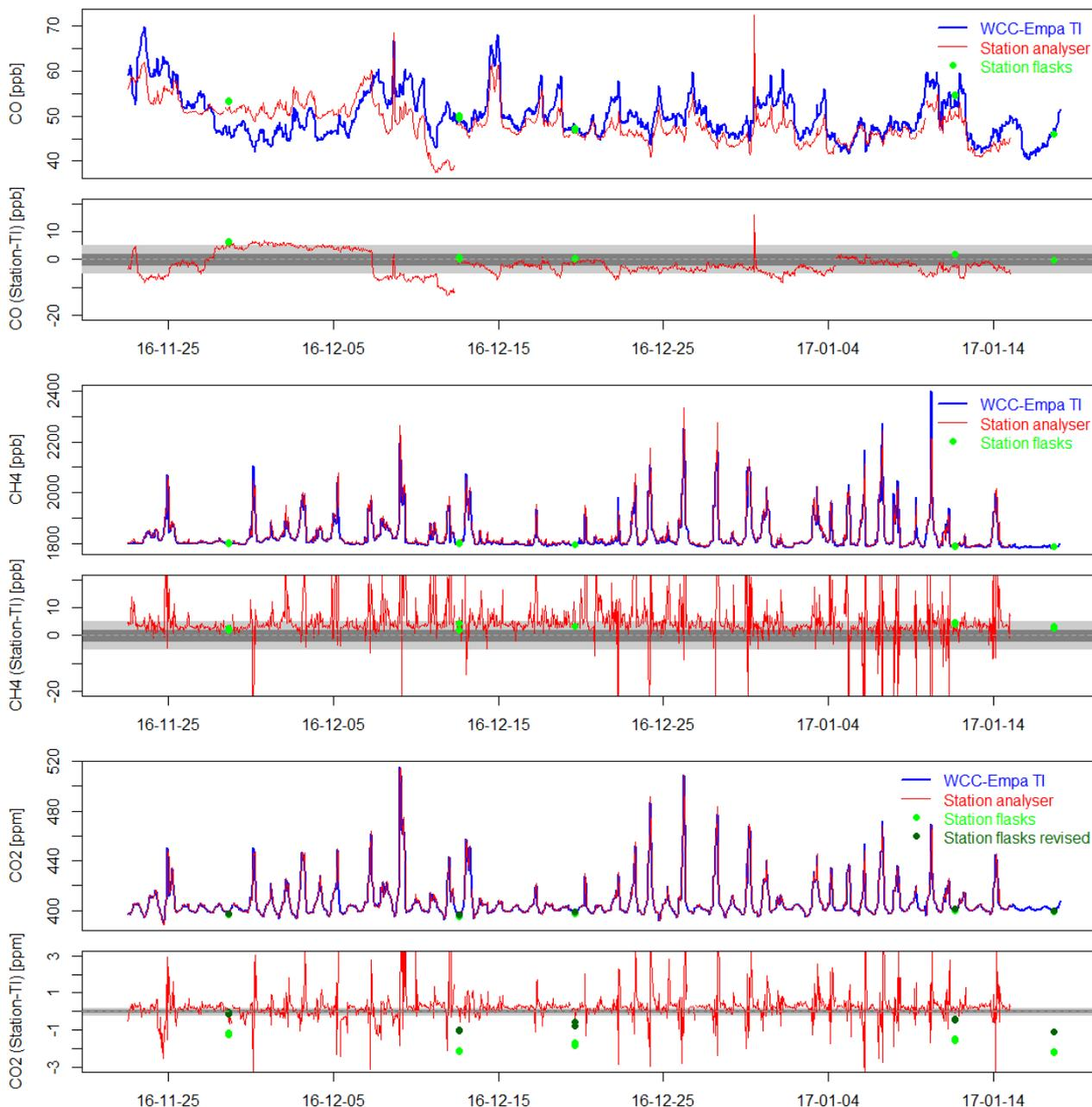
**Figure 12.** Comparison of the LAU IFTS analyser with the WCC-Empa travelling instrument for CO (top), CH<sub>4</sub> (middle) and CO<sub>2</sub> (bottom). LAU flask measurements are shown as green dots. Time series based on hourly data as well as the difference between the IFTS and the TI is shown. The horizontal grey areas correspond to the WMO/GAW compatibility (dark grey) and extended compatibility (light grey) goals.
