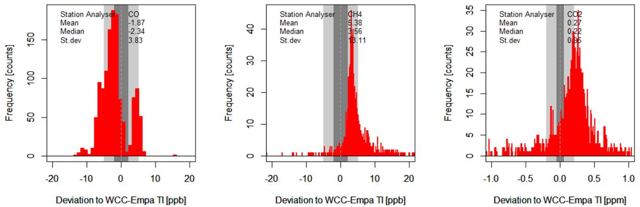
**Figure 13.** Deviation histograms for the LAU IFTS analyser for CO (left), CH<sub>4</sub> (middle) and CO<sub>2</sub> (right). 1 h data is shown for the station analyser – TI.
