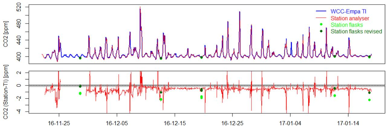
**Figure 14.** Comparison of the LAU NDIR CO<sub>2</sub> analyser with the WCC-Empa travelling instrument. Time series based on hourly data as well as the difference between the IFTS and the TI is shown. The horizontal grey areas correspond to the WMO/GAW compatibility (dark grey) and extended compatibility (light grey) goals.
