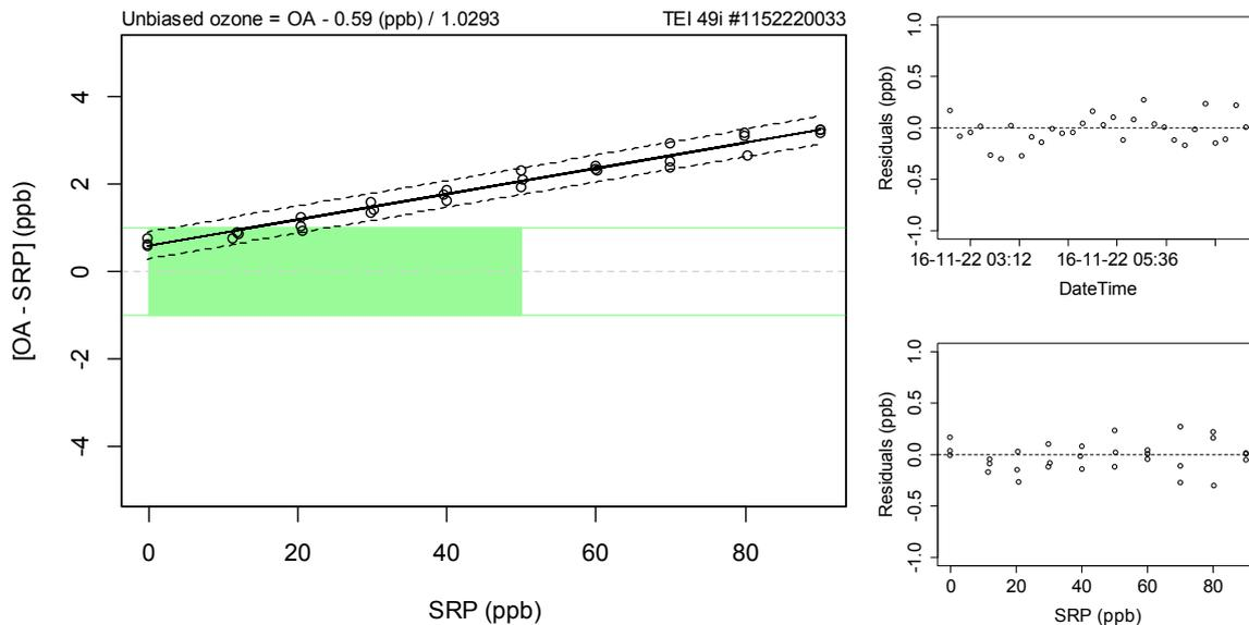
**Figure 3.** Same as above for the future BHD ozone analyser with initial (factory) calibration settings (Thermo Scientific 49C #01152220033).
