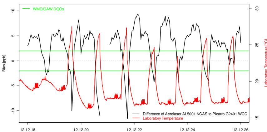
**Figure 10.** Bias of the NCAS Aerolaser AL5001 compared to the Picarro G2401 for a selected period and laboratory air temperature.
