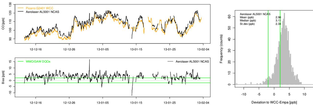
**Figure 9.** Upper left panel: CO time series (hourly averages) measured at CVO with the Picarro G2401 travelling instrument and the Aerolaser AL5001 analyser of NCAS. Lower left panel: Deviation of the NCAS system compared to the travelling instrument. Right panel: Frequency distribution of the deviations. The green lines refer to the WMO/GAW DQOs.
