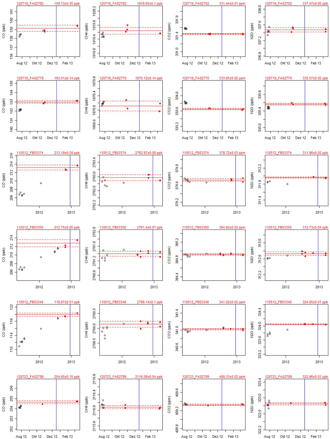
**Figure 17.** Results of the WCC-Empa TS calibrations. Only the values of the red solid circles were considered for averaging. The red solid line is the average of the points that were considered for the assignment of the values; the red dotted line corresponds to the standard deviation of the measurement. The blue horizontal line refers to the date of the audit.
