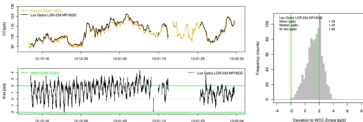
**Figure 11.** Upper left panel: CO time series (hourly averages) measured at CVO with the Picarro G2401 travelling instrument and the Los Gatos LGR-23d analyser of MPI-BGC. Lower left panel: Deviation of the MPI-BGC system compared to the travelling instrument. Right panel: Frequency distribution of the deviations. The green lines refer to the WMO/GAW DQOs.
