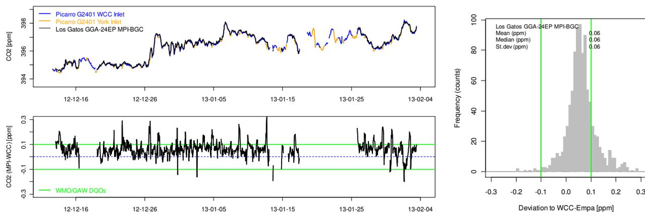
**Figure 13.** Upper left panel: CO<sub>2</sub> time series (hourly averages) measured at CVO with the Picarro G2401 travelling instrument and the Los Gatos GGA-24EP system of MPI-BGC. Lower left panel: Deviation of the MPI-BGC system compared to the travelling instrument. Right panel: Frequency distribution of the deviations. The green lines refer to the WMO/GAW DQOs.
