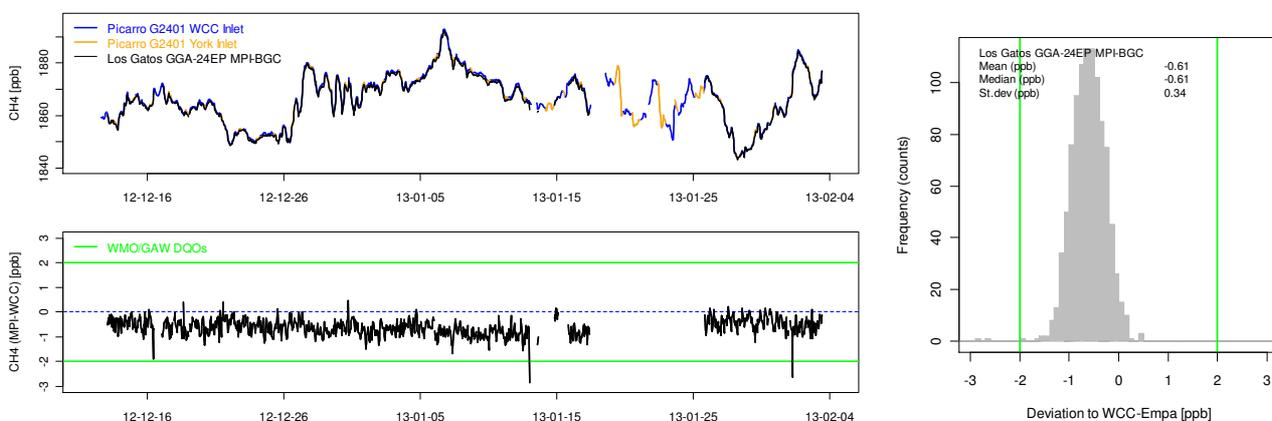
**Figure 12.** Upper left panel: CH<sub>4</sub> time series (hourly averages) measured at CVO with the Picarro G2401 travelling instrument and the Los Gatos GGA-24EP system of MPI-BGC. Lower left panel: Deviation of the CVO system compared to the travelling instrument. Right panel: Frequency distribution of the deviations. The green lines refer to the WMO/GAW DQOs.
