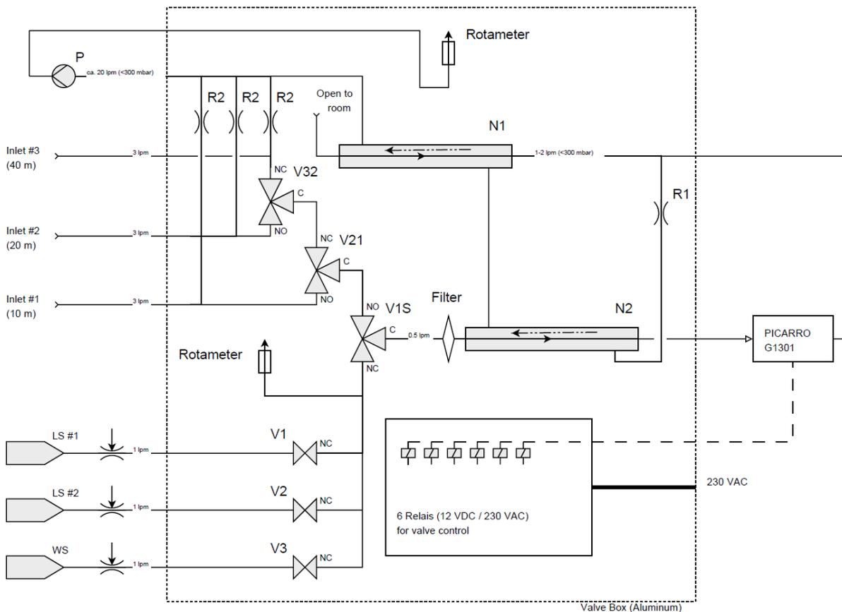
**Figure 13.** Picarro G1301 set-up at BKT.
