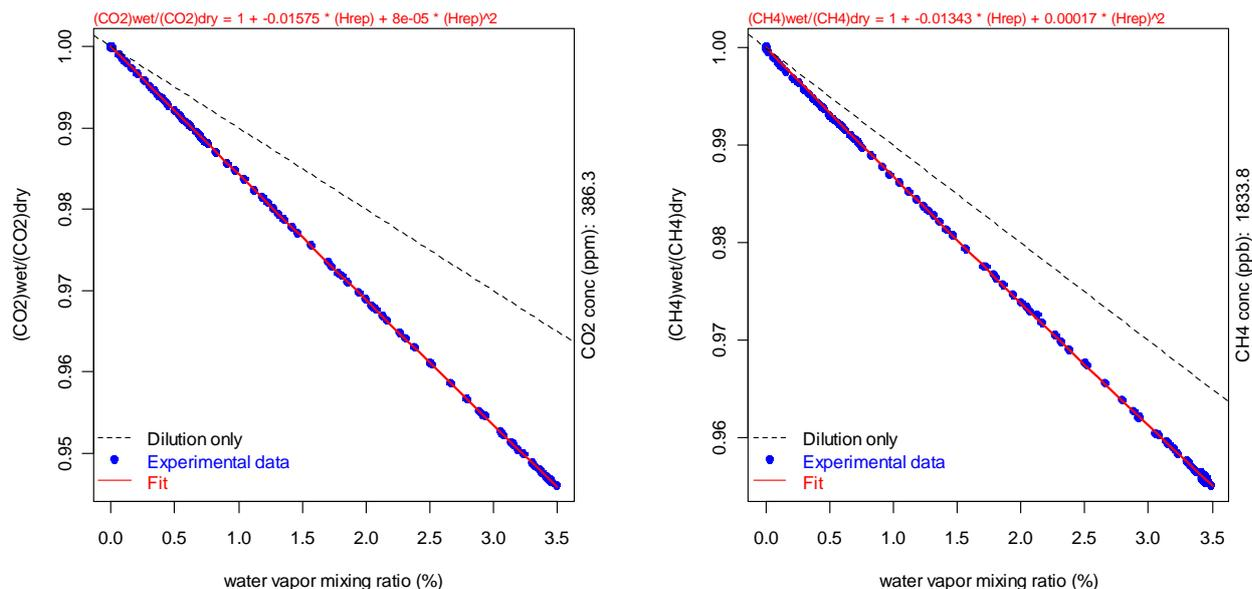
**Figure 14.** Quadratic fits for the BKT Picarro G1301 instrument of CO<sub>2</sub>wet/CO<sub>2</sub>dry and CH<sub>4</sub>wet/CH<sub>4</sub>dry vs. H<sub>2</sub>O mixing ratios.
