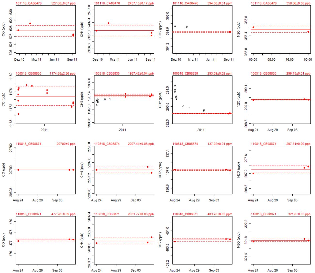
**Figure 16.** Results of the WCC-Empa TS calibrations. The red solid line is the average of the points that were considered for the assignment of the values; the red dotted line corresponds to the standard deviation of the measurement.
