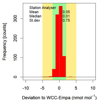
**Figure 14.** Carbon monoxide deviation histograms for the ZSF LGR 913-0015-1000 analyser.
