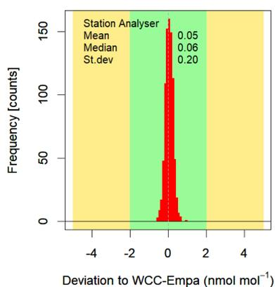
**Figure 16.** Methane deviation histogram for the ZSF Picarro G2301.
