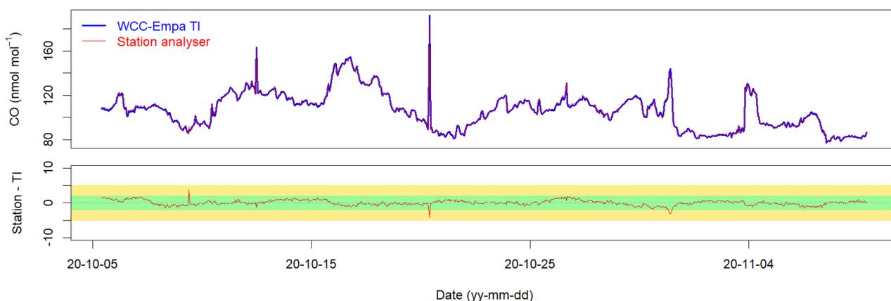
**Figure 13.** Comparison of the LGR 913-0015-1000 analyser with the WCC-Empa travelling instrument for CO. Time series based on hourly data as well as the difference between the station instrument and the TI is shown. The coloured horizontal areas correspond to the WMO/GAW compatibility (green) and extended compatibility (yellow) goals.
