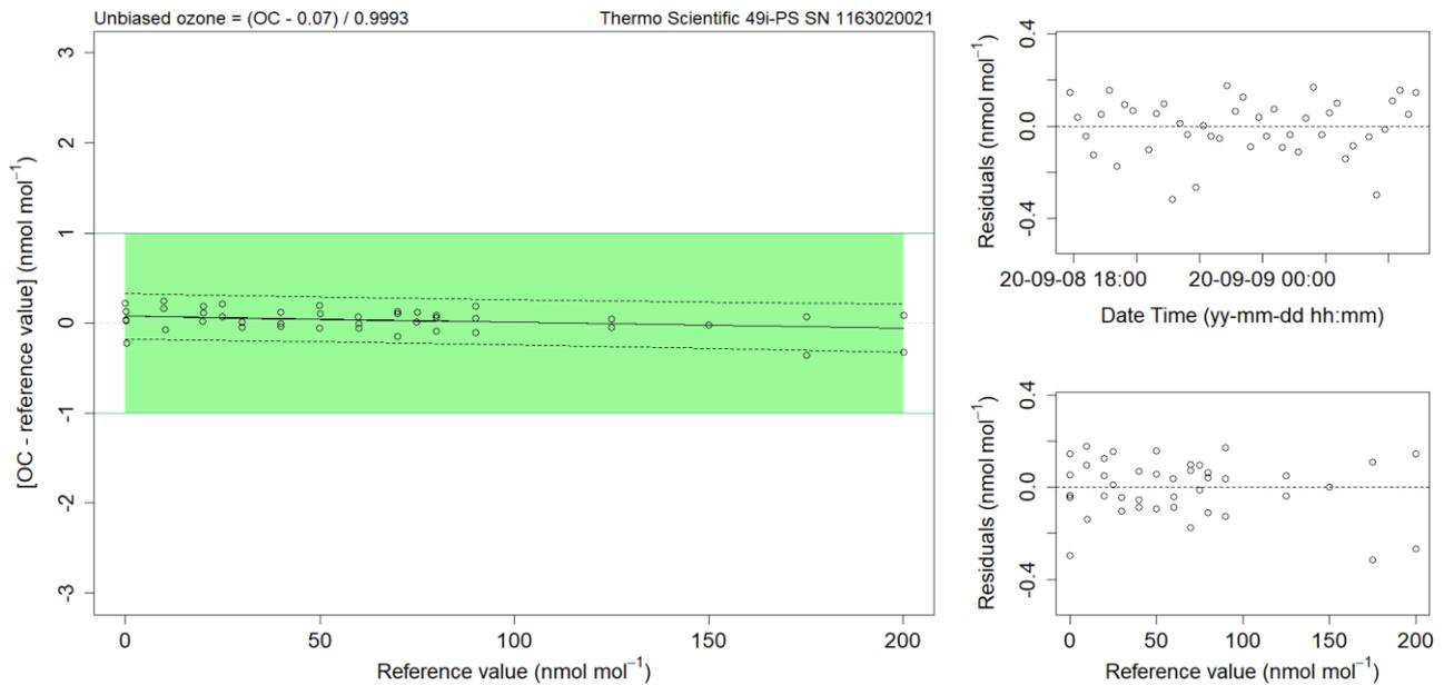
**Figure 2.** Same as above for the ZSF Thermo Scientific 49i-PS #1163020021 ozone calibrator (uncorrected, data as measured by the instrument were used for the comparison).
