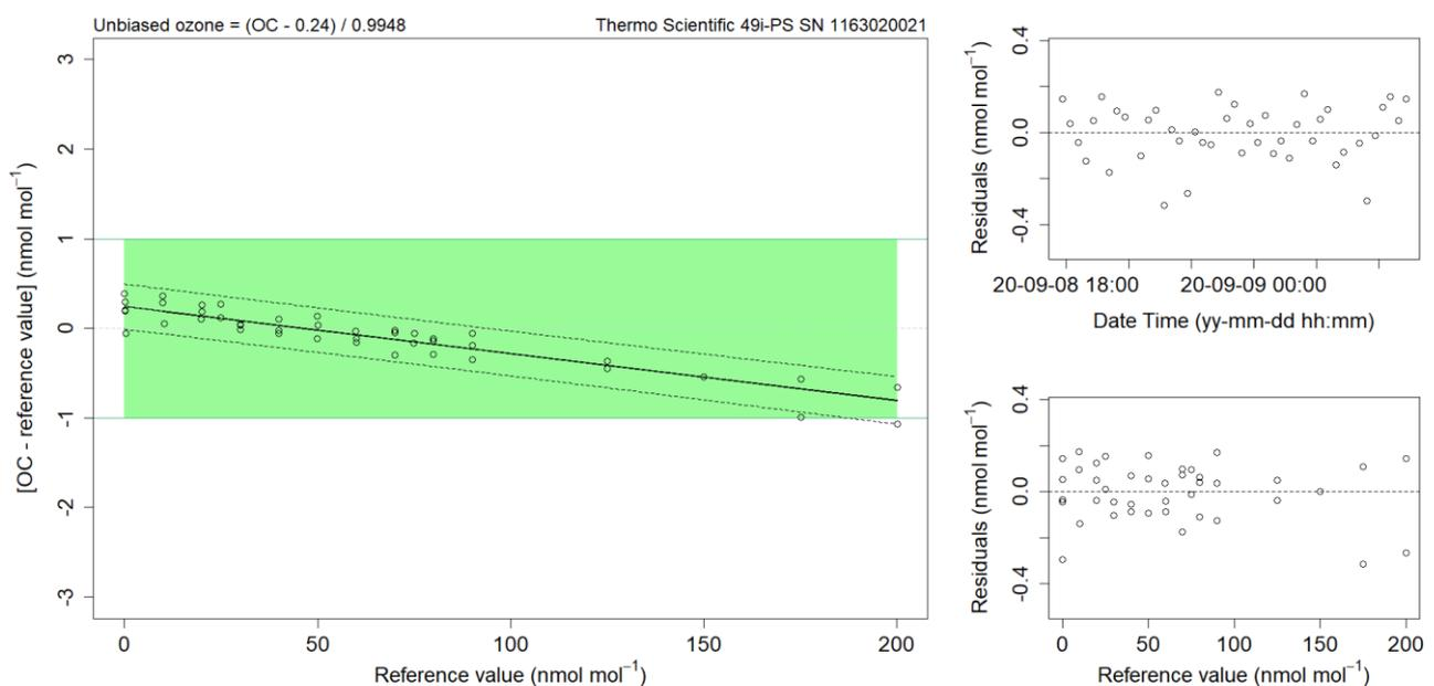
**Figure 3.** Same as above for the ZSF Thermo Scientific 49i-PS #1163020021 ozone calibrator (corrected based on calibration certificate from UBA Langen from 18. February 2020).
