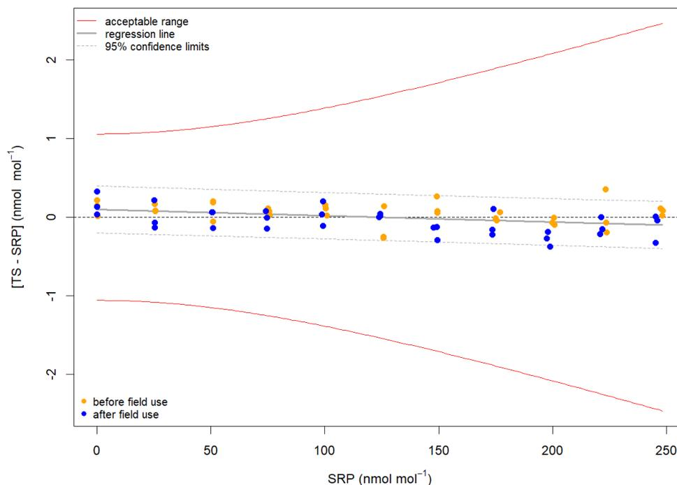
**Figure 31.** Deviations between traveling standard (TS) and Standard Reference Photometer (SRP) before and after use of the TS at the field site.
