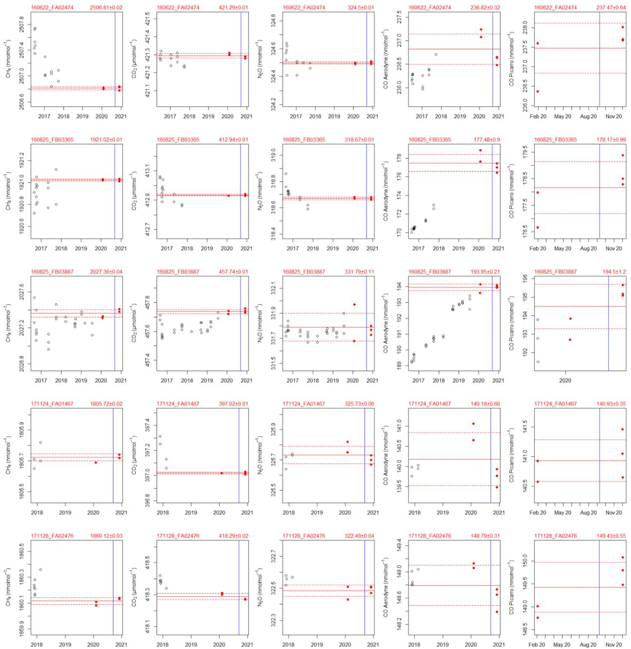
**Figure 32.** Results of the WCC-Empa TS calibrations. Only the values of the red solid circles were considered for averaging. The red solid line is the average of the points that were considered for the assignment of the values; the red dotted line corresponds to the standard deviation of the measurement. The blue vertical line refers to the date of the audit.
