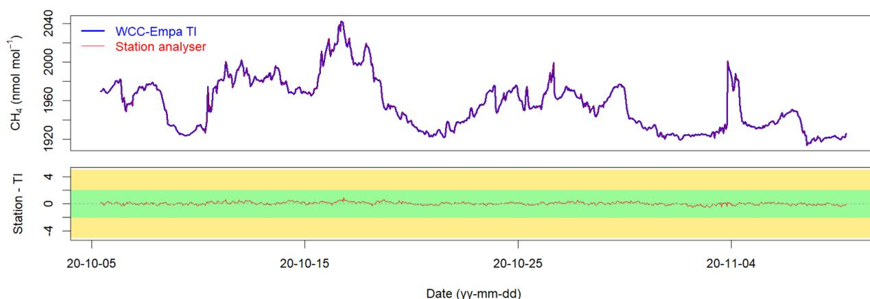
**Figure 15.** Comparison of the ZSF Picarro G2301 with the WCC-Empa travelling instrument for  $\text{CH}_4$ . Time series based on hourly data as well as the difference between the station instrument and the TI is shown. The coloured horizontal areas correspond to the WMO/GAW compatibility (green) and extended compatibility (yellow) goals.
