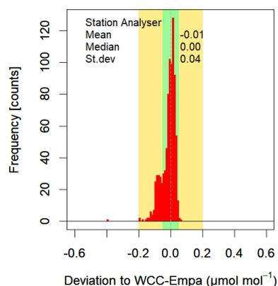
**Figure 18.** Carbon dioxide deviation histogram of the ZSF Picarro G2301 compared to WCC-Empa.
