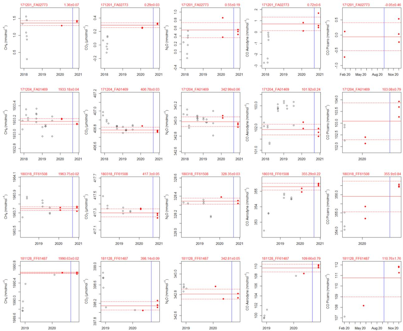
**Figure 33.** Results of the WCC-Empa TS calibrations. Only the values of the red solid circles were considered for averaging. The red solid line is the average of the points that were considered for the assignment of the values; the red dotted line corresponds to the standard deviation of the measurement. The blue vertical line refers to the date of the audit.
