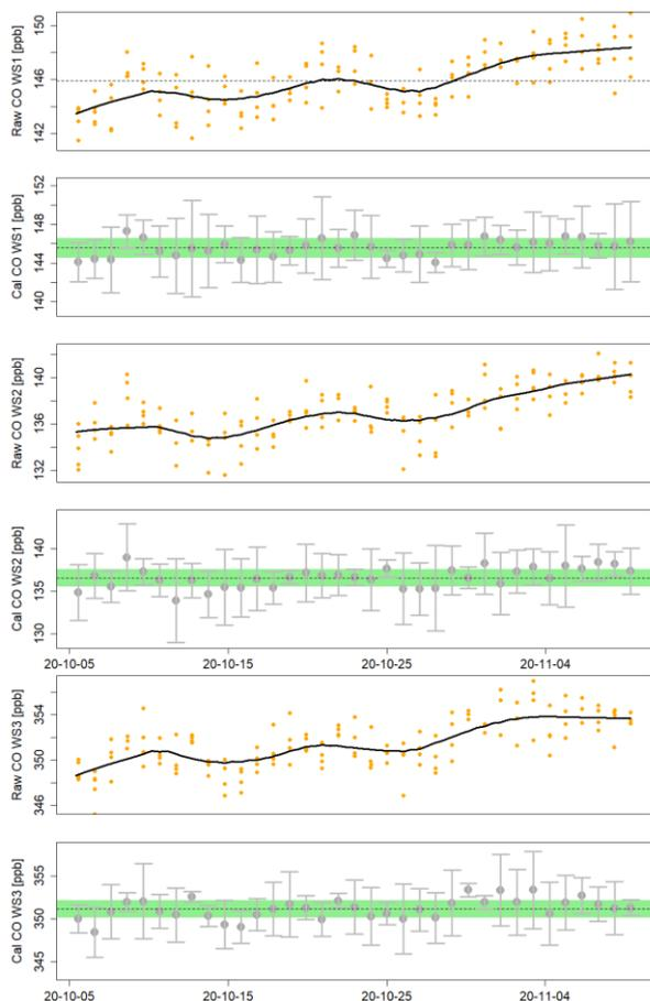
**Figure 34.** CO calibrations of the instrument used for the ambient air. The panels with the orange dots show raw 1 min values of the working standards and the loess fit (black line) used to account for drift. The other panels show the variation of the WS after applying the drift correction. Individual points in these panels are 5 min averages, and the error bars represent the standard deviation. The green area represents half of the WMO/GAW compatibility goals.
