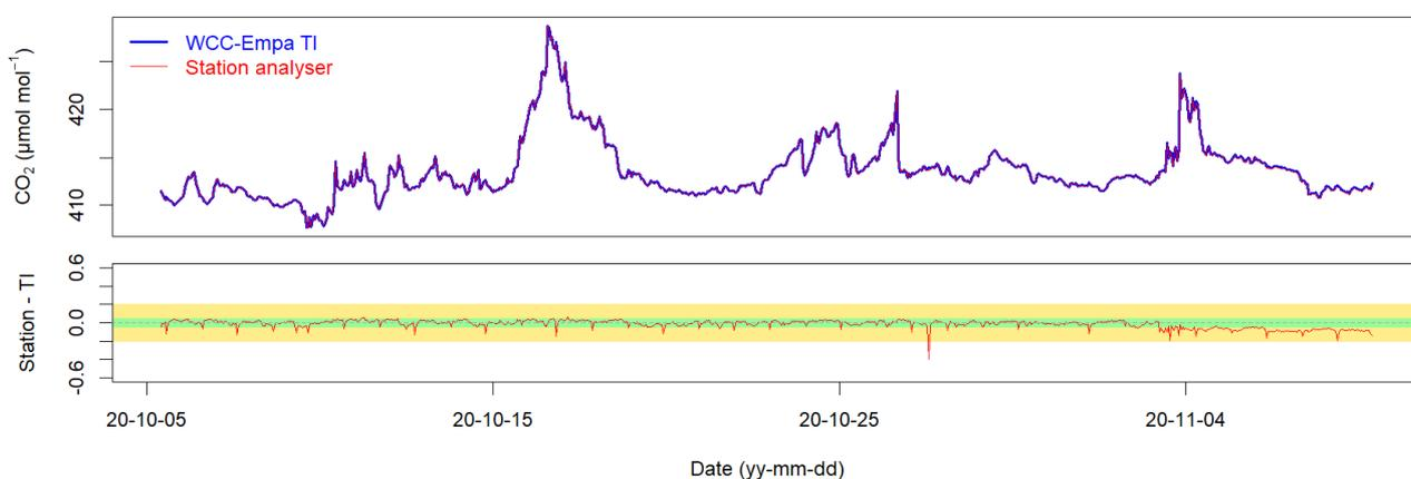
**Figure 17.** Comparison of the ZSF Picarro G2301 with the travelling instrument for CO<sub>2</sub>. Time series based on hourly data as well as the difference between the station instrument and the TI is shown. The coloured horizontal areas correspond to the WMO/GAW compatibility (green) and extended compatibility (yellow) goals.
