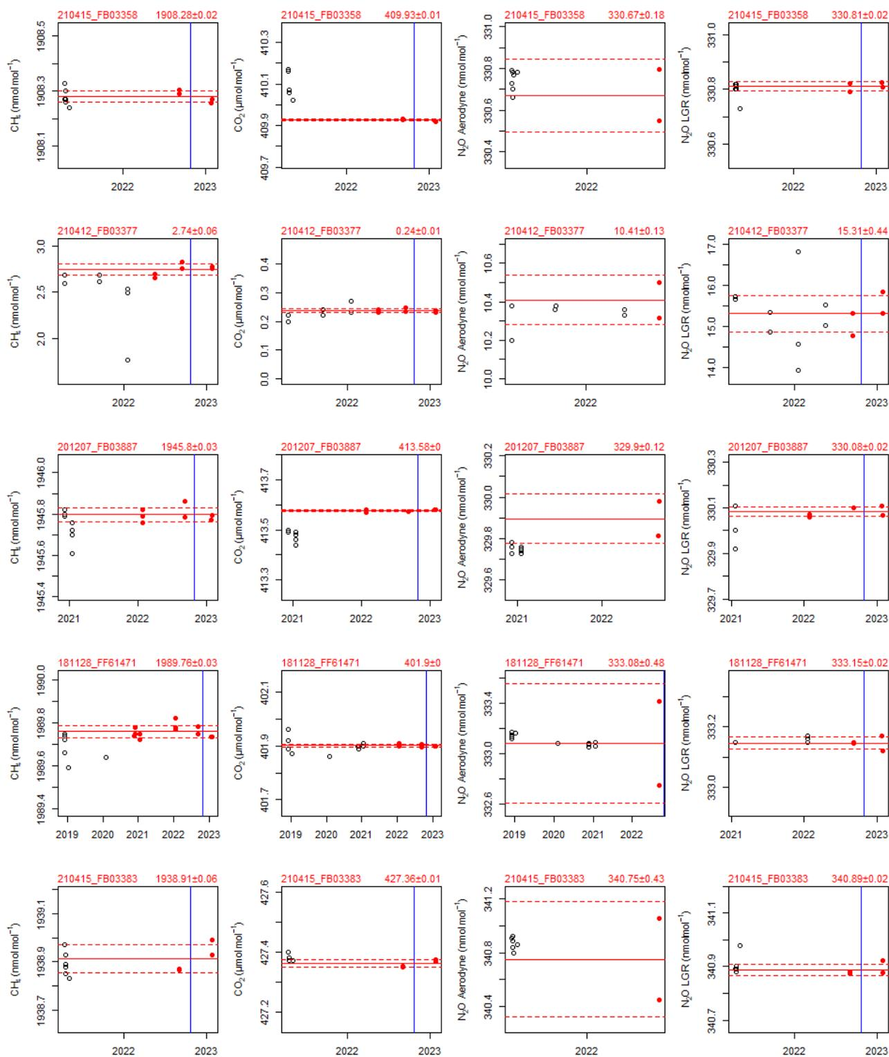
**Figure 16.** Results of the WCC-Empa TS calibrations for CH<sub>4</sub>, CO<sub>2</sub>, and N<sub>2</sub>O. Only the values of the red solid circles were considered for averaging. The red solid line is the average of the points used to assign the values; the red dashed line corresponds to the standard deviation of the measurement. The blue vertical line refers to the date of the audit.
