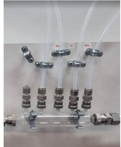
*Manifold of the reactive gases inlet.*
