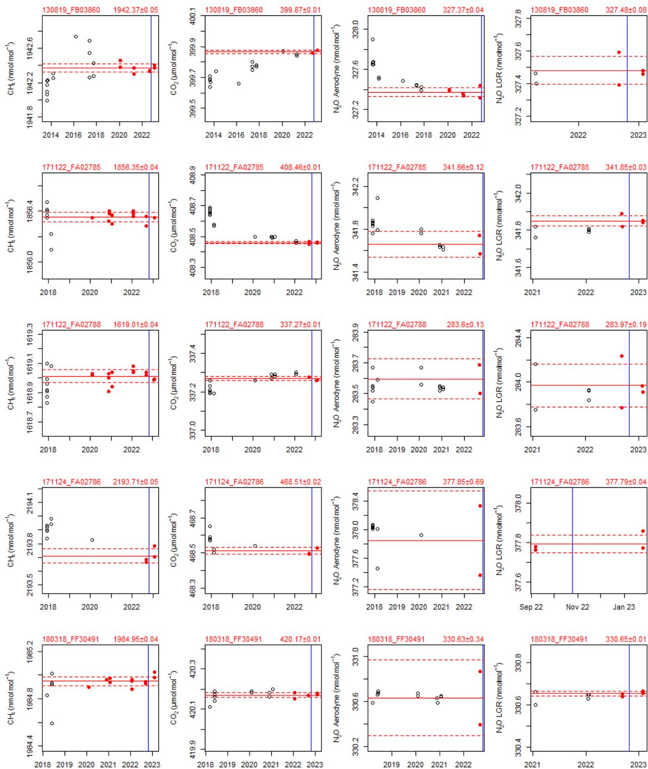
**Figure 15.** Results of the WCC-Empa TS calibrations for  $\text{CH}_4$ ,  $\text{CO}_2$ , and  $\text{N}_2\text{O}$ . Only the values of the red solid circles were considered for averaging. The red solid line is the average of the points used to assign the values; the red dashed line corresponds to the standard deviation of the measurement. The blue vertical line refers to the date of the audit.
