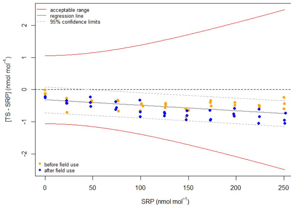
**Figure 14.** Deviations between TS and SRP before and after use of the TS in the field.
