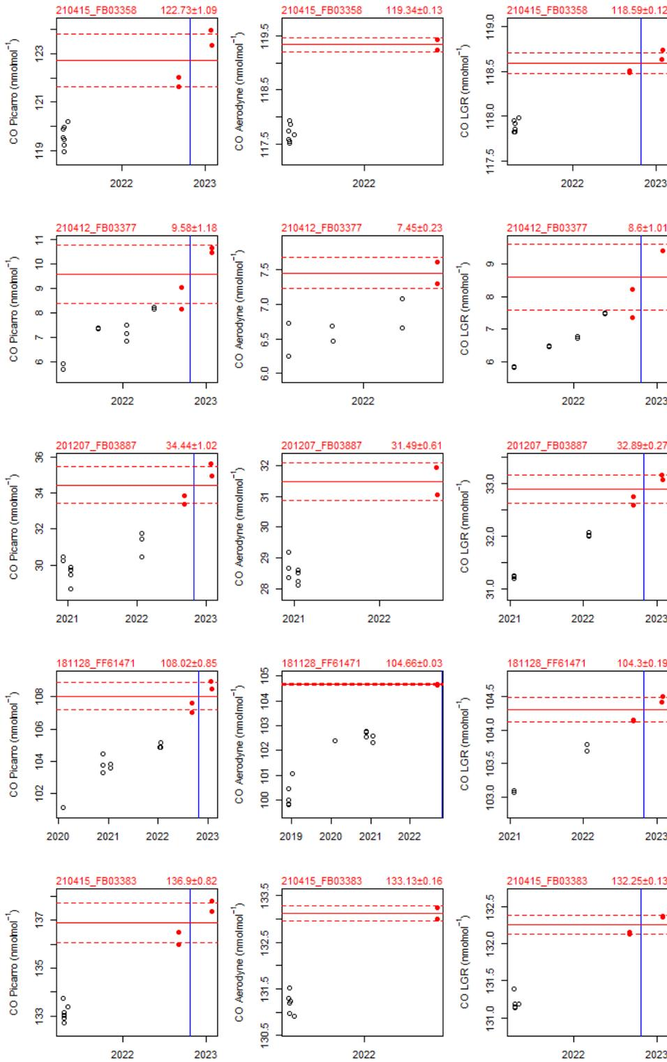
**Figure 18.** Results of the WCC-Empa TS calibrations for CO. Only the values of the red solid circles were considered for averaging. The red solid line is the average of the points used to assign the values; the red dashed line corresponds to the standard deviation of the measurement. The blue vertical line refers to the date of the audit.
