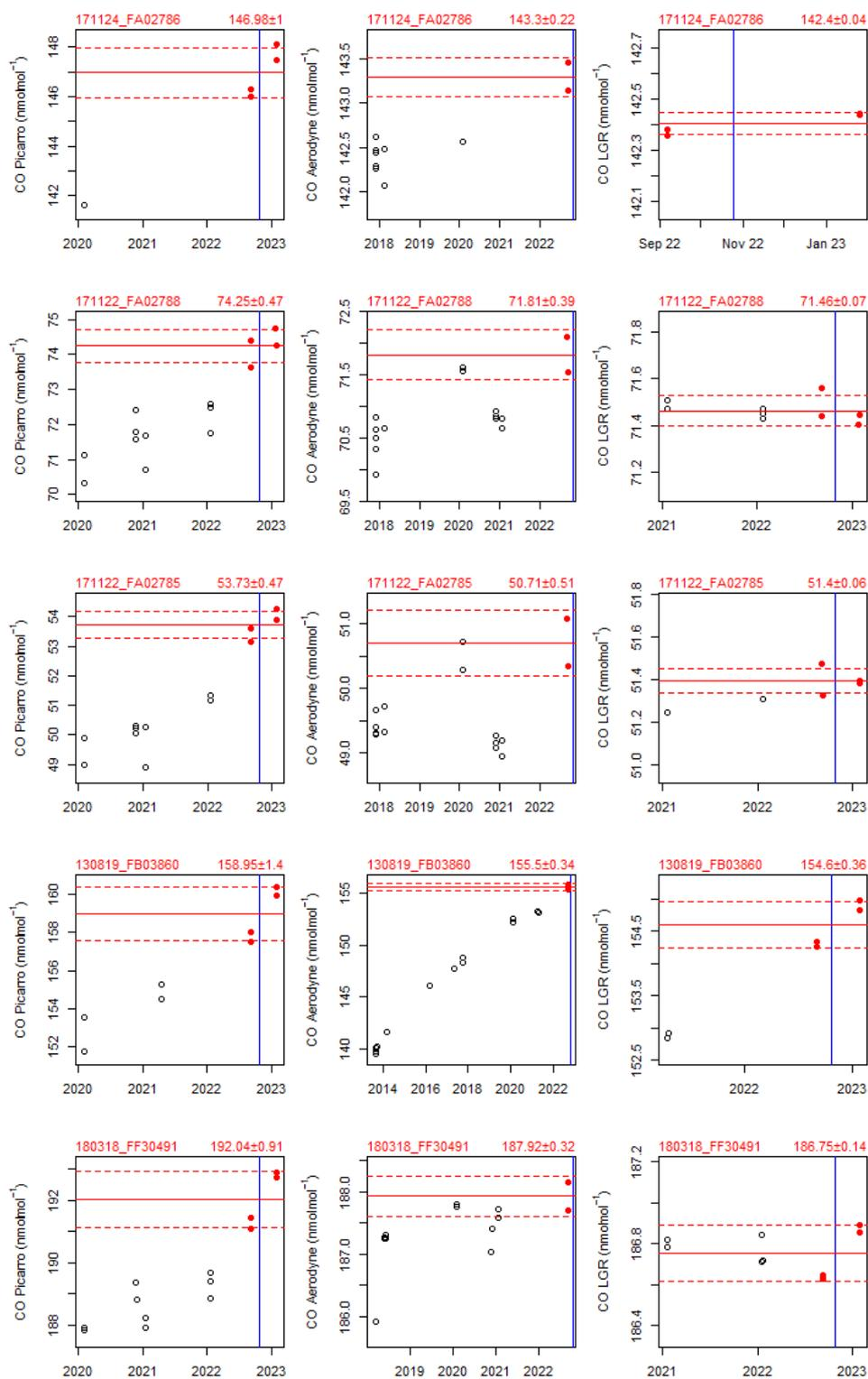
**Figure 17.** Results of the WCC-Empa TS calibrations for CO. Only the values of the red solid circles were considered for averaging. The red solid line is the average of the points used to assign the values; the red dashed line corresponds to the standard deviation of the measurement. The blue vertical line refers to the date of the audit.
