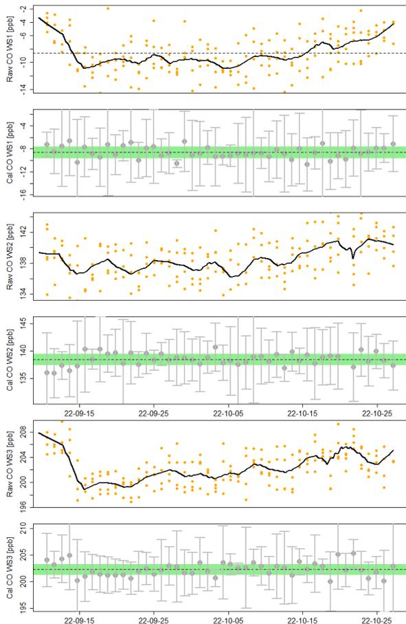
**Figure 20.** CO calibrations of the WCC-Empa-TI. The panels with the orange dots show the raw 1 min values of the working standards and the loess fit (black line) used to account for the drift. The other panels show the variation of the WS after application of the drift correction. Individual points in these panels are 5 min averages, and the uncertainty bars represent the standard deviation. The green area represents half of the WMO/GAW compatibility goals.
