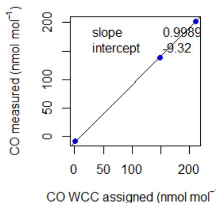
**Figure 21.** CO calibration function based on the average values of the drift corrected working standard measurements.
