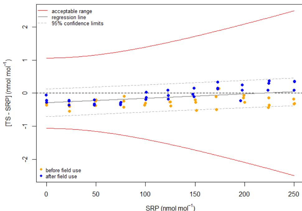
**Figure 14.** Deviations between traveling standard (TS) and Standard Reference Photometer (SRP) before use of the TS at the field site.
