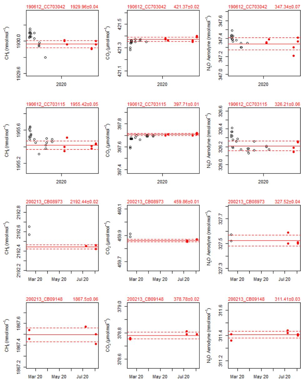
**Figure 15.** Results of the WCC-Empa TS calibrations for CH<sub>4</sub>, CO<sub>2</sub>, and N<sub>2</sub>O. Only the values of the red solid circles were considered for averaging. The red solid line is the average of the points that were considered for the assignment of the values; the red dotted line corresponds to the standard deviation of the measurement. The blue vertical line refers to the date of the audit.
