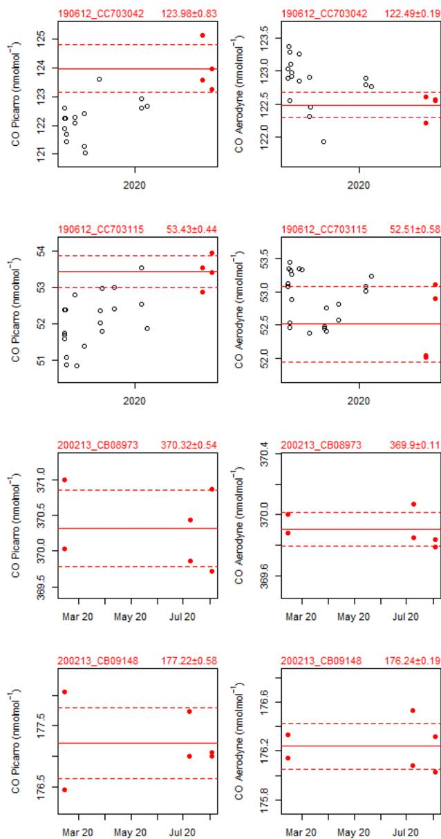
**Figure 16.** Results of the WCC-Empa TS calibrations for CO. Only the values of the red solid circles were considered for averaging. The red solid line is the average of the points that were considered for the assignment of the values; the red dotted line corresponds to the standard deviation of the measurement. The blue vertical line refers to the date of the audit.
