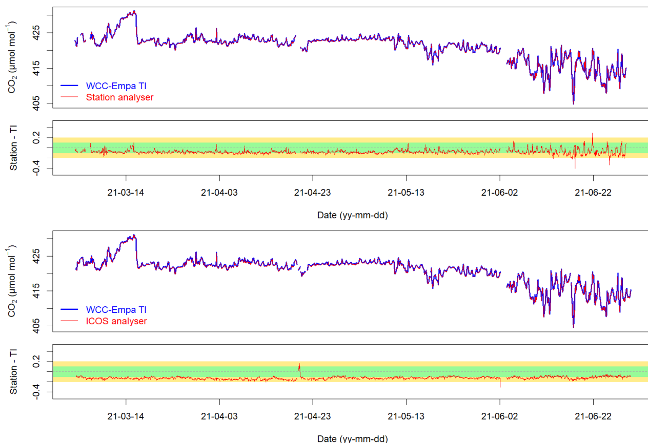
Figure 13. Comparison of the PAL Picarro G2401 G2401#306-CFKADS-2066 (instrument without dryer) (top) and the Picarro G2401#2037-CFKADS2164 (instrument with dryer) (bottom) with the WCC-Empa travelling instrument for CO 2 . Time series based on hourly data and the difference of the station instrument to the TI are shown. The coloured horizontal areas correspond to the WMO/GAW compatibility (green) and extended compatibility (yellow) goals.
