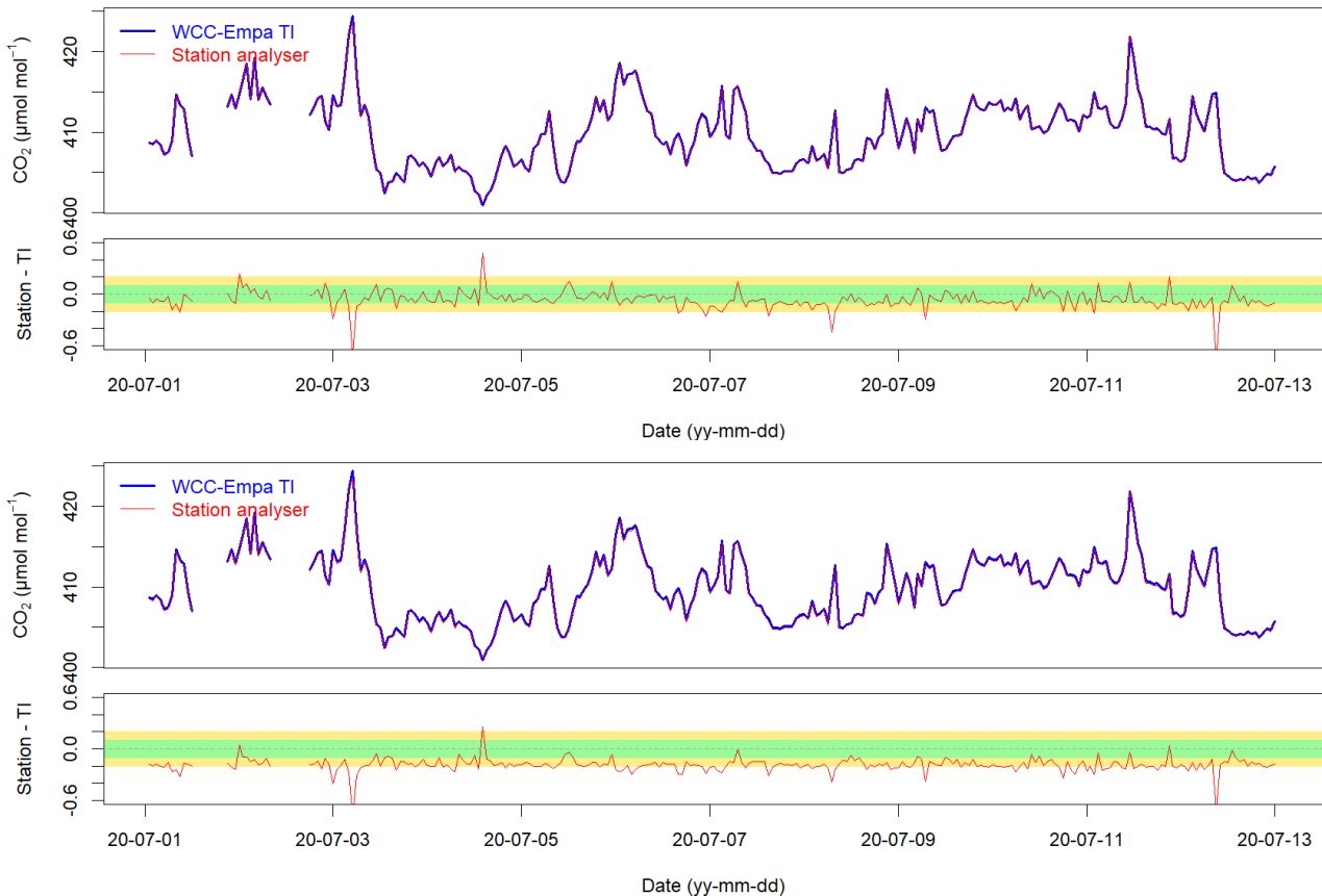
Figure 22. Comparison of the HPB Picarro G2401 G2401#1670-CFKADS2120 (top) and the Picarro G2401#2322-CFKADS2192 (bottom) with the WCC-Empa travelling instrument for CO 2 . Time series based on hourly data as well as the difference between the station instrument and the TI is shown. The coloured horizontal areas correspond to the WMO/GAW compatibility (green) and extended compatibility (yellow) goals.
