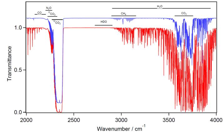
**Fig. 1.** The mid-infrared absorption spectrum of clean air in a 24 m cell. Red: undried air, blue: dried air. Positions of main absorption Griffith et al., 2012
