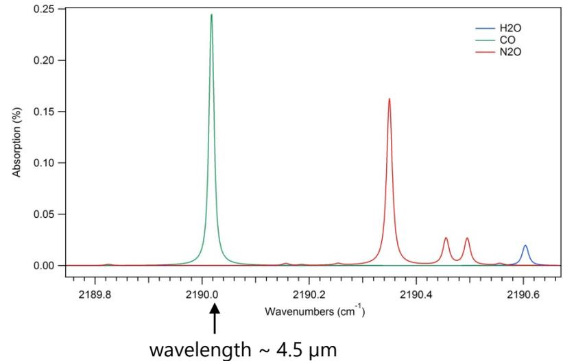
CO is detected in the near to mid-infrared region
