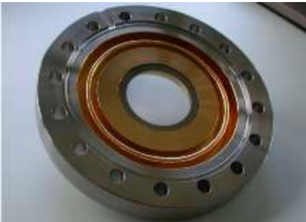
CVD diamond window in UHV flange
