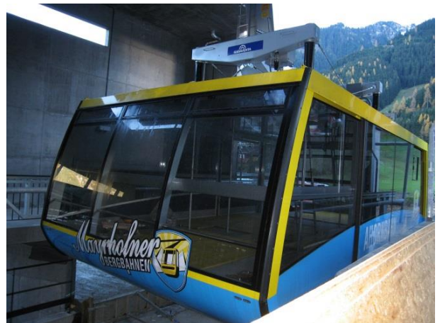
Teleferic cabin: RSGs applied to the traveling and suspension gear, and cabin (160 persons). Mayrhof im Zillertal, Austria.
