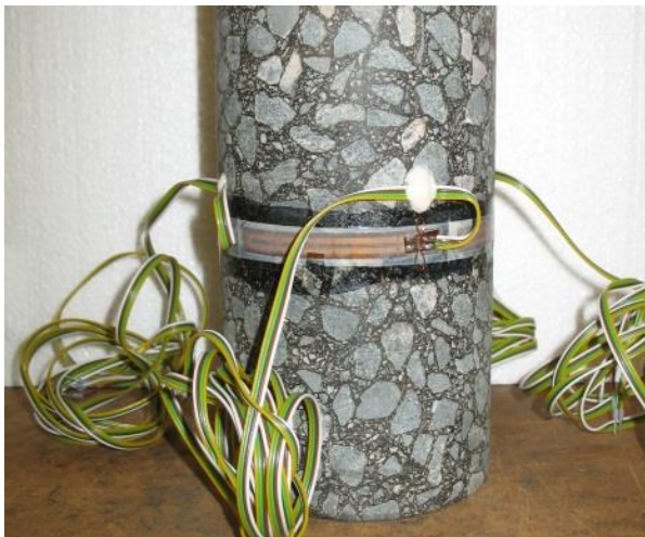
Road construction: Drill core sample equipped with 100 mm RSG for measuring hoop strains in compression.
