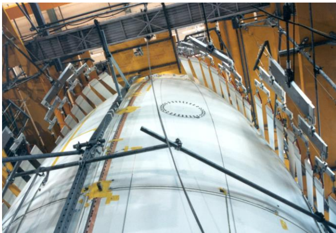
Ariane 5: Payload fairing during tension and pressure testing at Empa.
