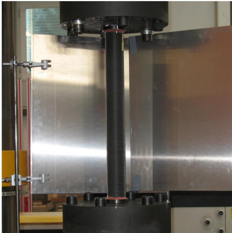
Set-up with mirrors for 360° monitoring
