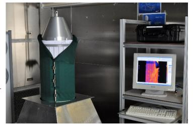
Elastic samples are often sewn into a tube with pre-set stretch level, whereas non-stretch samples are fixed on the main cylinder with clamps.
