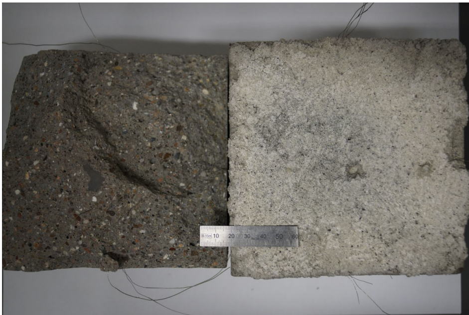
Figure 10. View of the heated surface of concrete cubes after the high-temperature spalling test. Left: sample without aerogel mortar, showing deep spalling. Right: sample with 48-mm thick aerogel mortar layer, without spalling.
