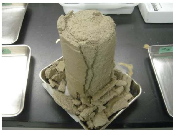
Figure 1: Severe damaged of cement solidified cylinder of MSWI-FA after 256 days dissolution.
