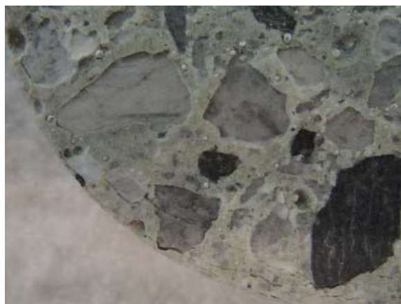
Figure 2: Paste expansion and cracking of normal concrete core immersed in concentrated solution from MSWI-FA at 5°C for 1 year.
