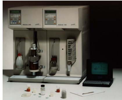
Figure 1: Mercury intrusion porosimeter
