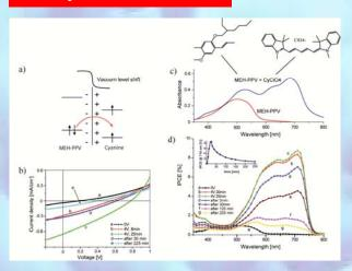
For as-prepared bilayer MEH-PPV / cyanine films, HOMO energies are close and charge transfer after photoexcitation of the cyanine is suppressed. (a) Displacing  $\text{ClO}_4^-$  (-) across the junction with an external voltage bias induces a potential energy shift and the device is "turned on". (b and d)  $\text{V}_{\text{oc}}$  and photocurrent response for different biasing and relaxation conditions. Effects are reproducible and reversible with a relaxation time of  $\sim 4~\text{h}$ .
