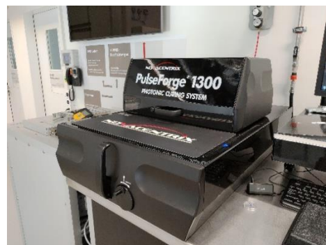
Flash lamp annealing machine PulseForge 1300 by Novacentrix at Empa.
