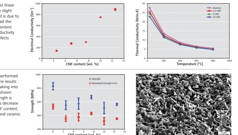
Three point bending strength tests were performed on bars of 1.7 x 2 x 20 mm dimension. The results were adjusted with a Weibull correction taking into account the small specimen size are also shown (20 x 3 x 2 mm). A 40 % decrease in strength is observed by the introduction of CNFs, this decrease in strength is stable up to 12.5 vol.% CNF content. Failure is due to a combination of CNFs and ceramic defects.
