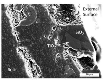
different corrosion products  $TiO_2$  and  $SiO_2$  in the  $Si_3N_4/TiN$ -AY composites,  $MoO_2$ ,  $SiO_2$  and  $Y_2Si_2O7$  in the  $Si_3N_4/MoSi_2$ -AY composites and  $Lu_2Si_2O_7$  and  $SiO_2$  in the  $Si_3N_4$ -L material.
