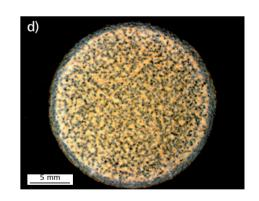
Exposure to oxidation and corrosion leads to the formation of a passive  ${\rm SiO_2}$  layer in the early stages. Further degradation is by diffusion of the environment through this layer. SEM studies showed the
