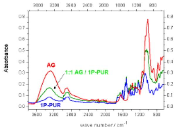
**Figure 1** IR-spectra of the hardened AG / 1P-PUR compound compared to AG and 1P-PUR
