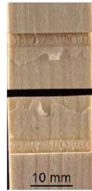
**Figure 5** Shear zone of spruce treated with 100 w.% AG; after aging treatment II
