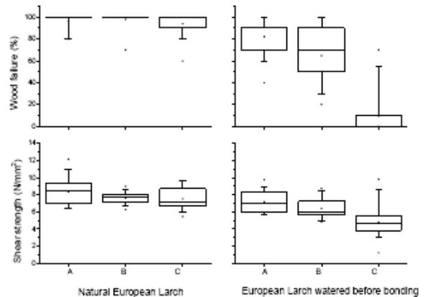
**Figure 9** Wood failure and shear strength of watered 1P-PUR bonded European larch wood samples (A Standard climate, B Treatment I, C Treatment II)
