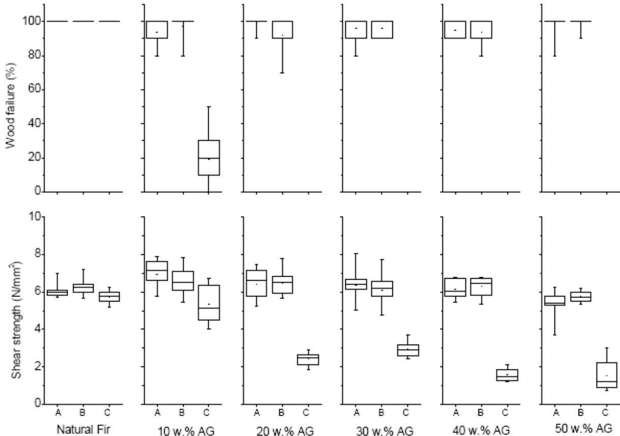
**Figure 3** Wood failure and shear strength of AG treated and IP-PUR bonded fir sample subsets after conditioning at 20%/65 % RH and the two aging treatments; only data test series 3 (A Standard climate, B Treatment I, C Treatment II)
