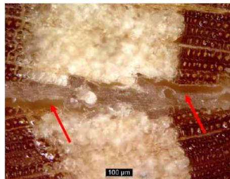
**Figure 10** Transverse section of a 1P-PUR bond line in European larch after treatment II; N.B. wood surface was treated with water before bonding
