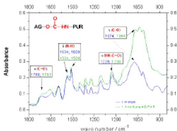
**Figure 2** IR-spectra of the hardened AG / 1P-PUR compound compared to 1P-PUR at the characteristic vibration bands of urethane
