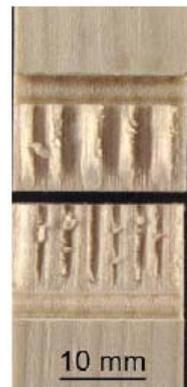
**Figure 4** Shear zone of untreated spruce with characteristic wood failure
