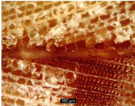
**Figure 12** Transverse section of a 1P-PUR bond line in European larch; wood surface was HMR primed before bonding
