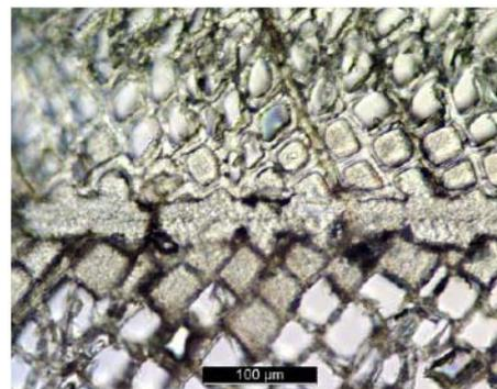
**Figure 6** Transverse section of 1P-PUR bonded fir after aging treatment II showing an intact bond line
