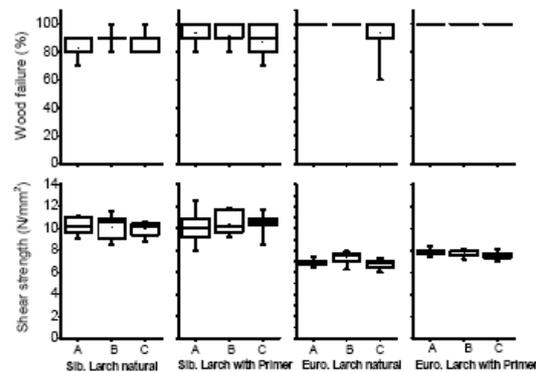
**Figure 11** Wood failure and shear strength of HMR primed, 1P-PUR bonded Siberian and European larch wood samples (A Standard climate, B Treatment I, C Treatment II)
