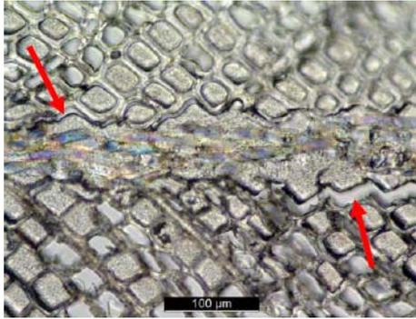
**Figure 7** Transverse section of a 1P-PUR bond line in fir after aging treatment II; wood were treated with 10 w.% AG before bonding
