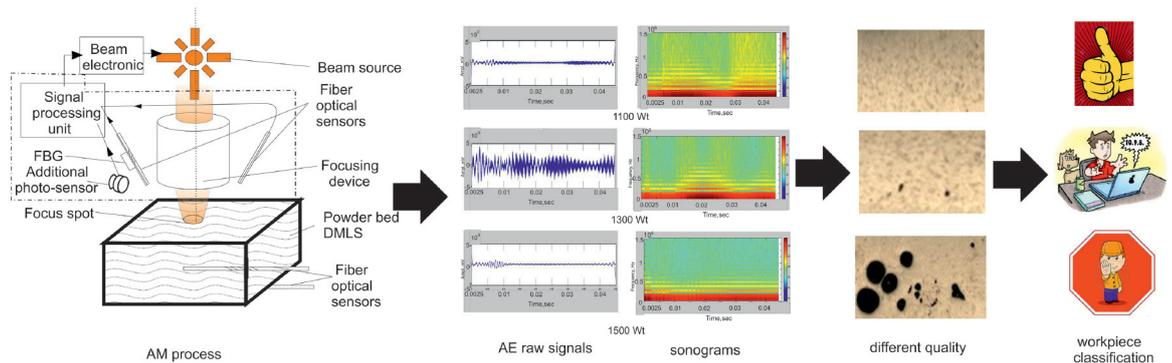
The advantages of this invention are twofold. First, the additive manufacturing process of a workpiece can be stopped as soon as the defined quality level is not reached, e.g. when there is porosity in the workpiece. Second, based on the measured signals, the process parameters can be optimized via a self-contained feedback control loop. Therefore, quality control and adaptation of subsequent process parameters are possible.
