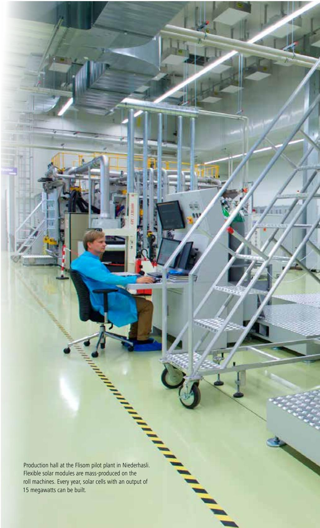
Production hall at the Flisom pilot plant in Niederhasli. Flexible solar modules are mass-produced on the roll machines. Every year, solar cells with an output of 15 megawatts can be built.
