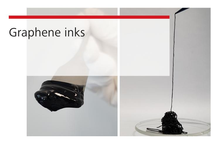
Additive-free graphene inks for printed electronics (2D) and structural elements (3D)
