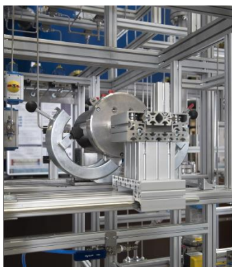
Fig 1. "Aerokinetics" apparatus at Hamburg University of Technology to determine the kinetics of supercritical drying
