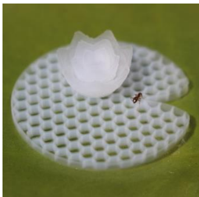
Fig 1 3D printing silica aerogel lotus flower
