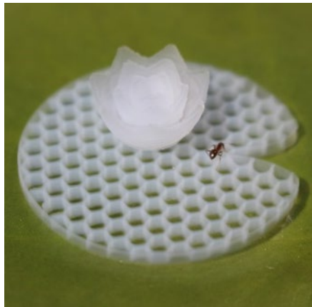
Fig 1. 3D printing silica aerogel lotus flower
