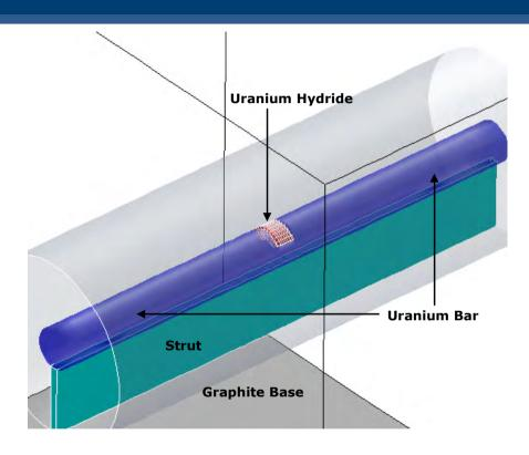
In the core, a single fuel channel is considered for the domain geometry.
