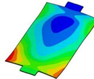
Mapping of results from forming shell FE-mesh using adaptivity to the fully integrated solid welding FE-mesh. The novel shell to solid mapping functionality in LS-PREPOST v4.2 is used.
