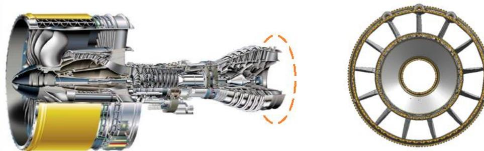
Load carrying 718 structure in the rear part of the GP7000 TEC engine.
