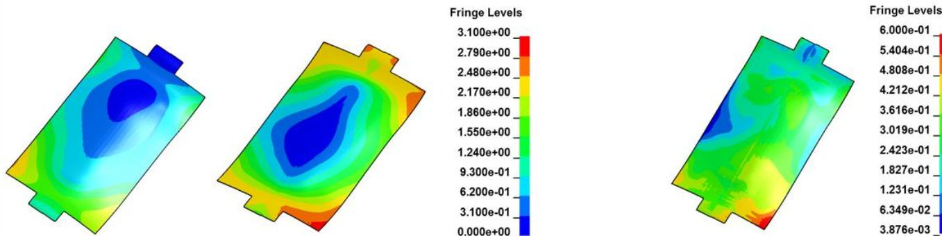
Part deviation after forming (left), welding (middle) and compensation (right), [mm]
