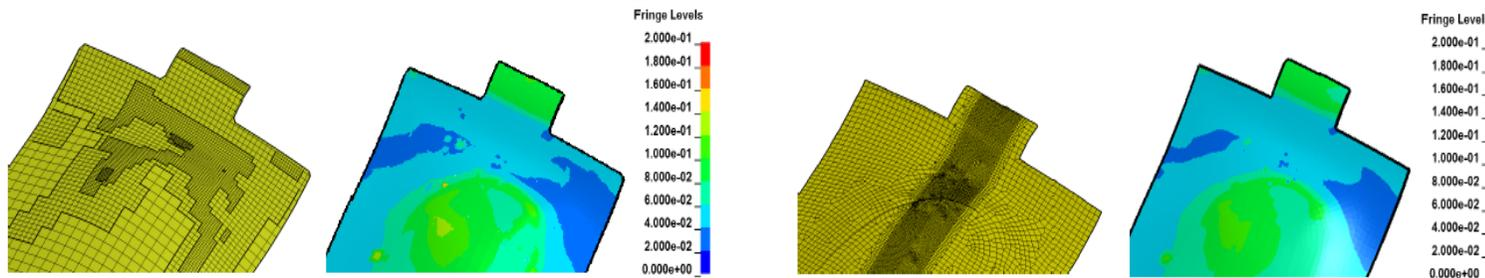
Forming simulation mesh (left) and welding simulation mesh (right) with mapping.
