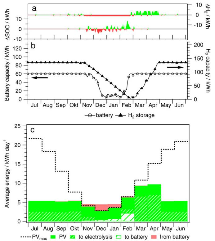
**Fig. 6.** Model C input analysis: (a) net energy flow to and from the battery and hydrogen storage as daily averages, (b) the evolution of absolute battery capacity and hydrogen capacity, and (c) energy per day as monthly averages. Fractions of PV production being used for battery charging and electrolysis are plotted as dashed areas.
