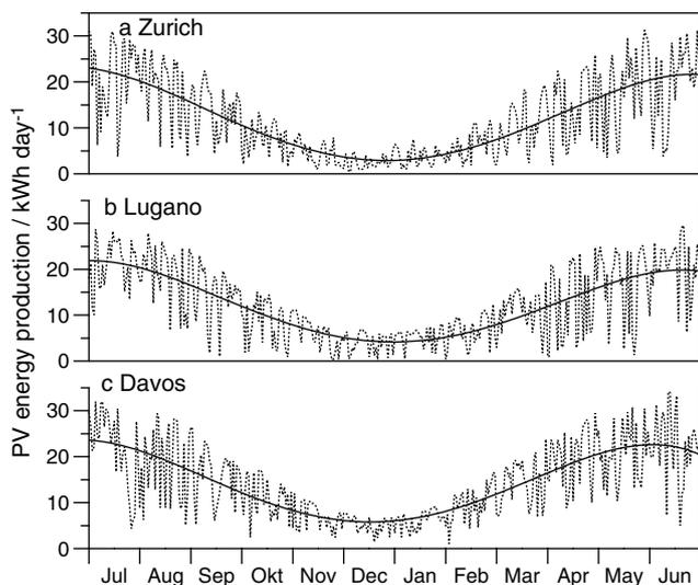
**Fig. 2.** PV production projections for locations specified in Table 2 based on actual solar data for SELF. The average daily production variations between summer and winter are: (a) 8:1, (b) 5:1, and (c) 4:1.
