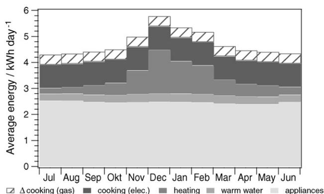
**Fig. 3.** The average energy demand per day for the individual services. The values represent average electrical energy for the respective service with the exception of cooking, where gas is applicable depending on the Model. Additional primary energy required for using gas vs. electricity is plotted separately.
