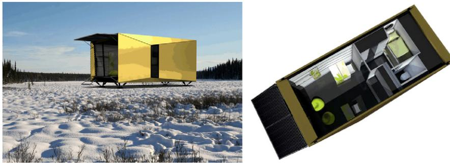
**Fig. 1.** The SELF stand-alone living unit. The size of the system is 3.5 m × 7.5 m × 3.2 m (W × L × H). The roof accommodates the PV system for energy production.
