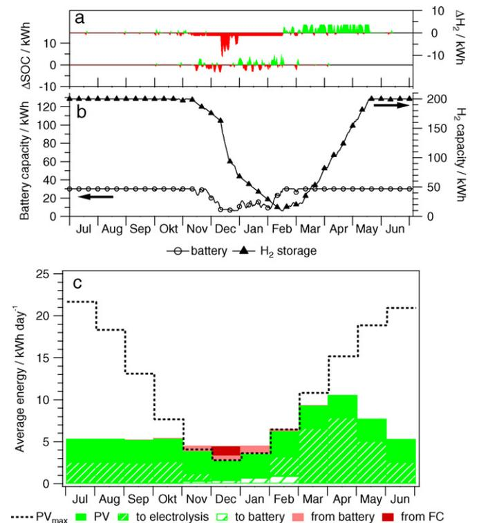
**Fig. 7.** Model D input analysis: (a) net energy flow to and from the battery and hydrogen storage as daily averages, (b) the evolution of absolute battery capacity and hydrogen capacity, and (c) energy per day as monthly averages.
