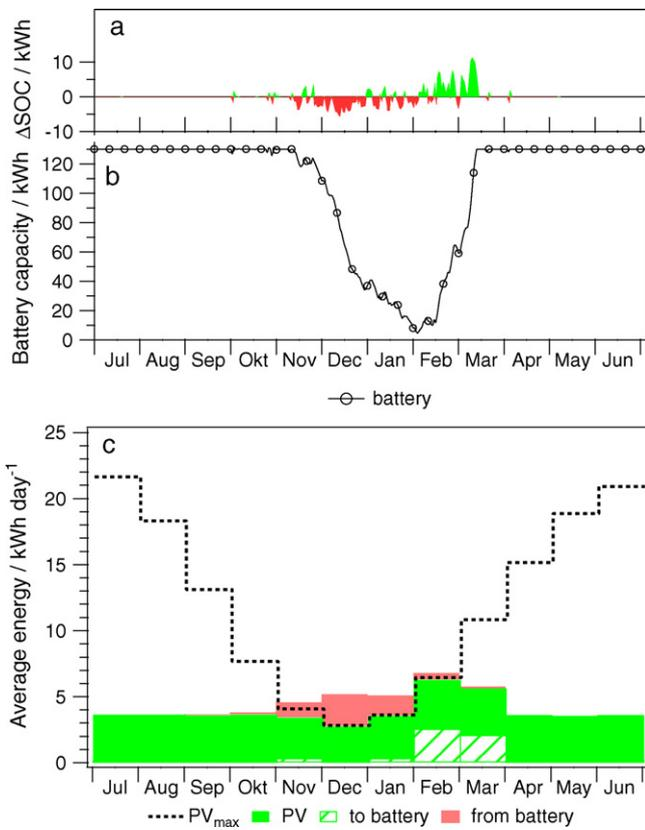
**Fig. 5.** Model B input analysis: (a) net energy flow to and from the battery as daily averages, (b) the evolution of absolute battery capacity, and (c) energy per day as monthly averages.
