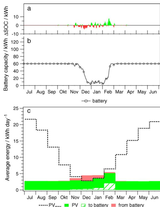
**Fig. 4.** Model A input analysis: (a) net energy flow to and from the battery as daily averages, (b) the evolution of absolute battery capacity, and (c) energy per day as monthly averages. “PV” represents the harvested share from the PV system. PV energy used to charge the battery is plotted as a dashed area while energy being sourced from the battery is marked in red as a stacked bar plot.
