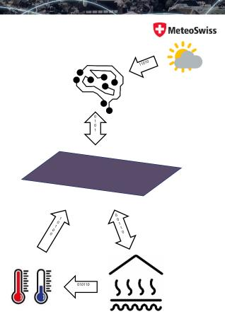
25% of heating and cooling energy can be saved with a predictive controller.
