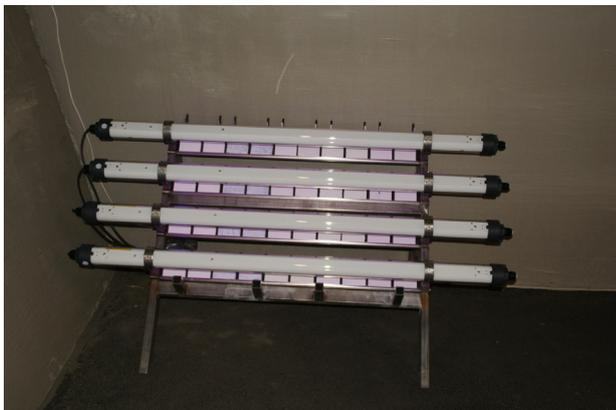
Figure 4. Samples placed in roadside Gallery with UV lamp system.
