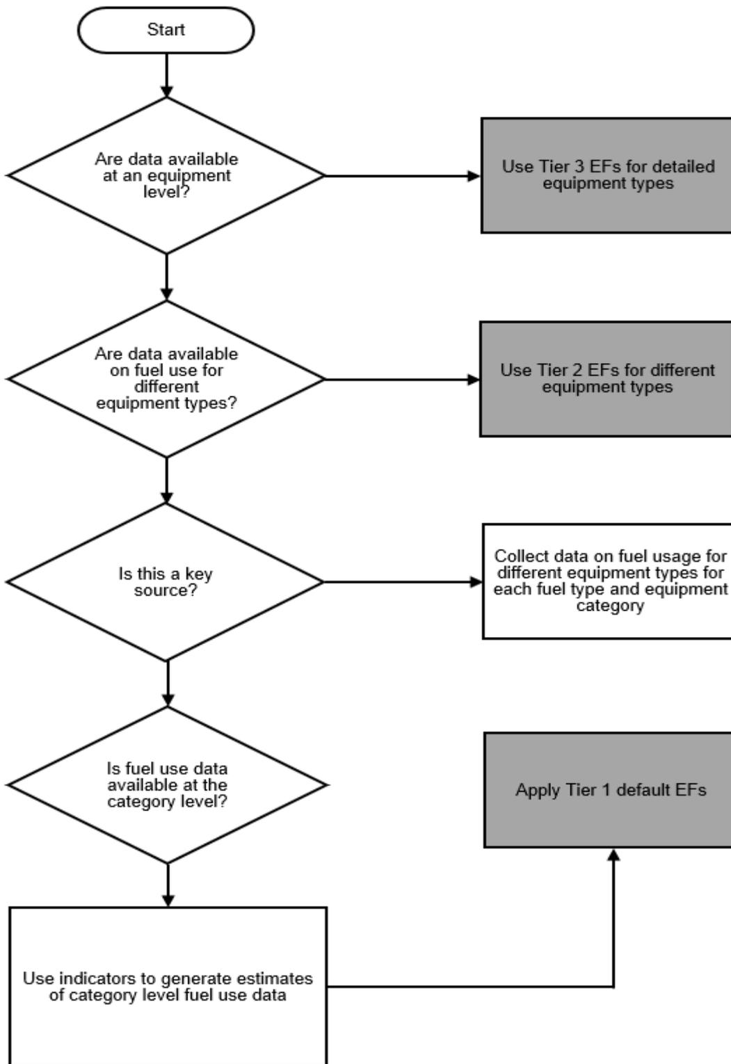
Figure 6. Decision tree for choosing method for calculating harmful emissions dependable about available data according to EMEP guide
