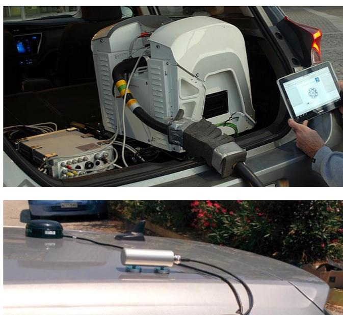
Figure 1: Up: The AVL GAS PEMS iS inside the trunk of the vehicle. Down: The GPS and ambient sensors on the roof of the vehicle.
