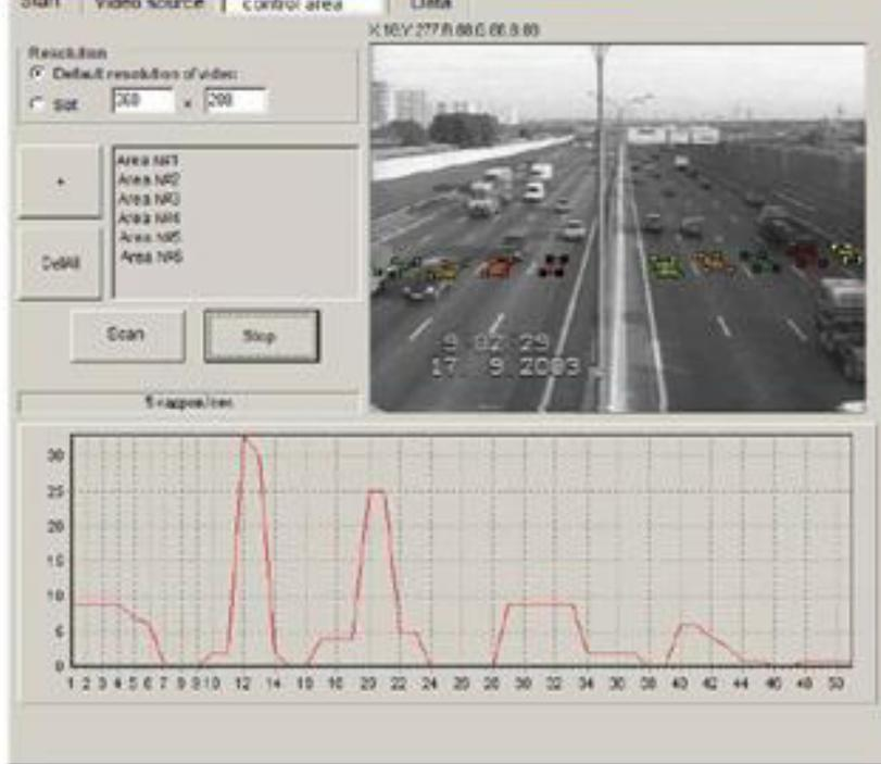
Figure 3. Method of virtual detectors
