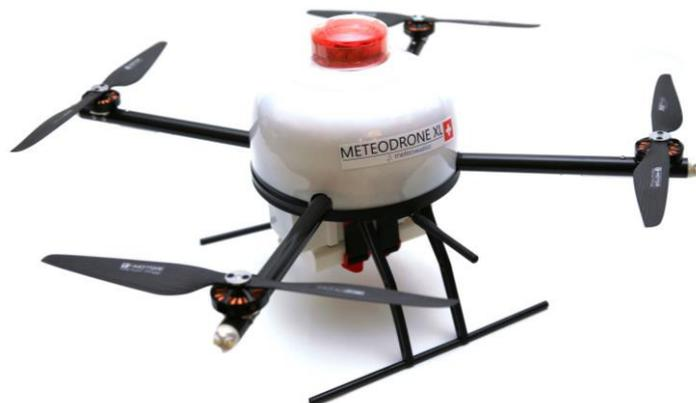
Figure 1: The MeteoDrone XL from Meteomatics AG used for measuring air pollution in the Misox Valley Switzerland case study.
