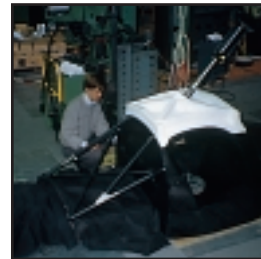
During filling with silage, selected locations (in this case the hatches) of an agricultural silo (height approx. 10 m, \phi approx. 4 m) are monitored using acoustic emission analysis.
