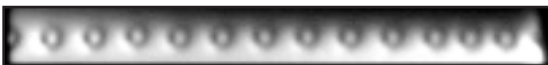
Eddy current amplitude image of drilled holes in a coated turbine blade
