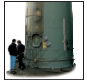
During filling with silage, selected locations (in this case the hatches) of an agricultural silo (height approx. 10 m, \phi approx. 4 m) are monitored using acoustic emission analysis.
