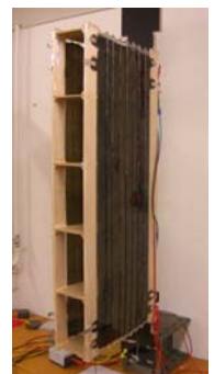
Figure 7: Active hinge for tail fin actuation
