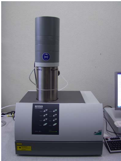
Figure 1: LFA 457 Microflash apparatus
