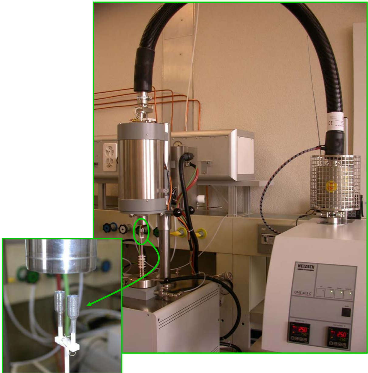
Figure 2: Thermogravimetric set up (TGA) coupled with the mass spectrometer (MS)
