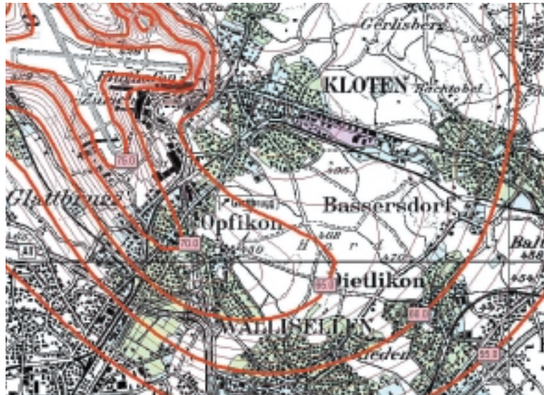
Fig. 1: Example of an aircraft noise calculation for Zurich airport. The red lines indicate the average noise loads L_{eq} in dB for the 16 hour period of the day.
