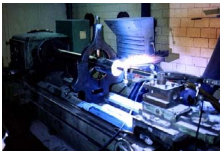
Fig. 15c: High pressure cylinder during internal coating.
