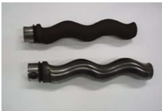
Fig. 15a: Slurry pump elements (top: as sprayed, bottom: finished)
