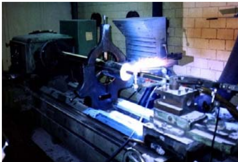
Fig. 4: Internal coating process carried out during the project for field tests.
