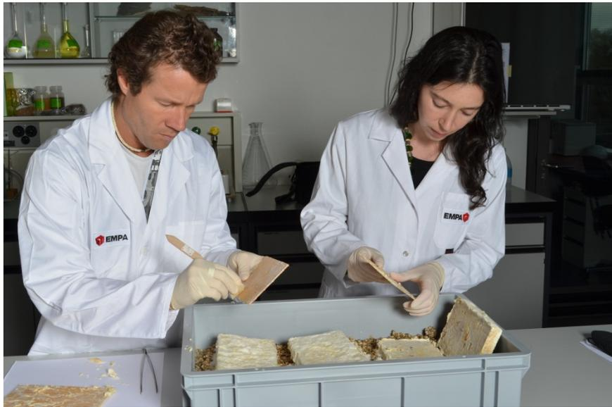
In the Biotechnology group of Empa Wood Lab, tonal woods are systematically treated with rot-inducing fungi. Markus Heeb and Iris Brémaud regularly check to see how the fungal attack is progressing.
