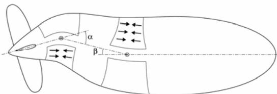
The EAPs merge into the airship hull at four points. When activated they expand, causing the hull to execute the “bending-rotation-stroke”, a technically simplified version of the motion of a fish in water.
