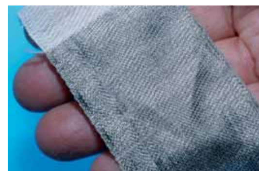
Fabric made of synthetic fiber coated with silver.
