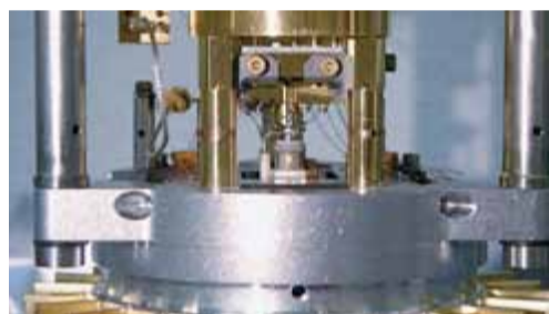
A look into the low-temperature scanning tunnel microscope (LT-STM), which operates at a temperature of 5 Kelvin (-268°C). The instrument operates at a temperature of 5 Kelvin, achieving a spatial resolution of about 0.01 nm and an energy discrimination of 5 meV.
