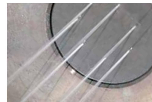
Multifilament spinneret. The liquid polymer is forced through the spinning nozzles at temperatures up to 300°C and a pressure of up to 100 bar. In this way a large number of bi-component fibres can be spun and processed simultaneously.
