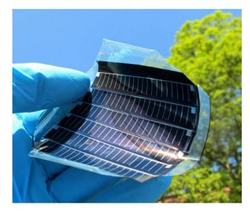
Fully monolithically integrated flexible solar module (consisting of 6 cells) based on cadmium telluride (CdTe): Empa researchers recently achieved a new world record in energy conversion efficiency of 13.8 percent with this type of solar cell.
